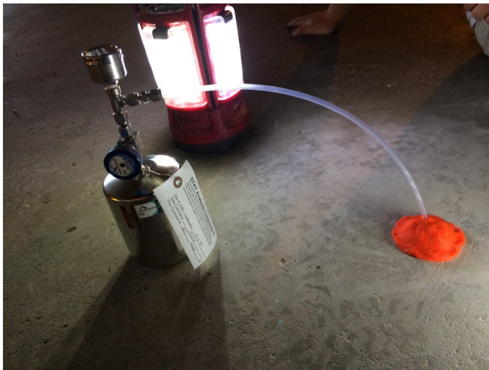
Photo 14. Summa canister screening sample collected from a sub-slab core hole sealed with non-toxic Play-Doh.
