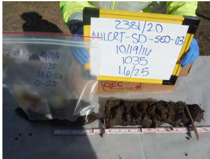
Photo Number: 1 Date of Photo: 10/17/16 Description: SED-03, Sand with Organic Fines
