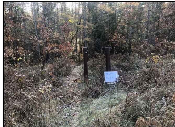
Monitoring Well MW4 and Piezometer MW4A Upon Inspection
