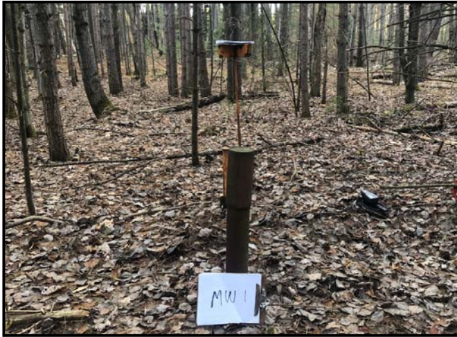
Monitoring Well MW1 Upon Inspection
