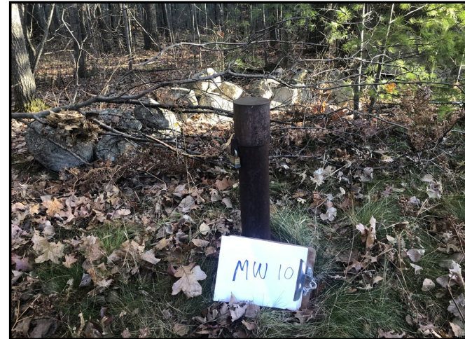
Monitoring Well MW10 Upon Inspection
