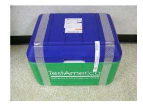
F. Close cooler, place signed and dated Custody Seals over opening. Tape over the Custody Seal and seal cooler securely. Fill out overnight shipping waybill and attach to the top or handle of the cooler. Attach Saturday delivery stickers if needed. Ship according to DOT regulations.
