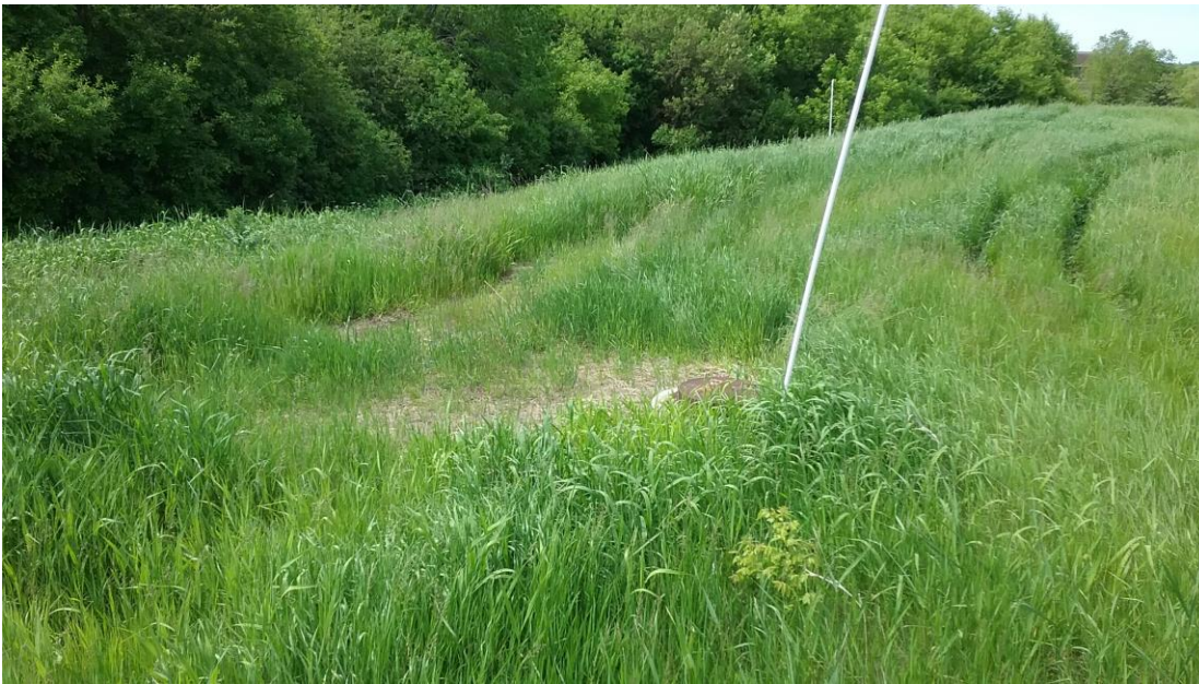
Photo #5: Gas Well EW-16 - Stressed Vegetation Surrounding Gas Well
