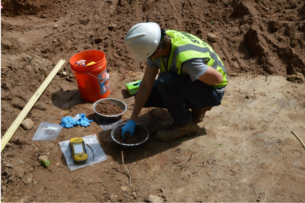
6/10/15: Collection of soil by consultant for five point composite sampling
