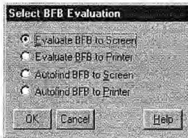
Figure 3. Choices for automated BFB tune evaluation by the EnviroQuant software. The "Evaluate BFB..." choices use the spectrum (single or averaged) in Data Analysis window 1 for evaluation. The "Autofind..." choices automatically find the BFB peak, average the top three BFB spectra and subtract a baseline spectrum prior to evaluation.
