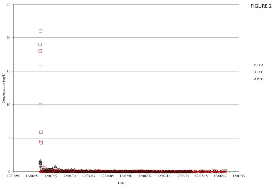
PRIMARY CHLORINATED VOCs IN THE MRDS SVE EXHAUST (ARITHMETIC SCALE)
