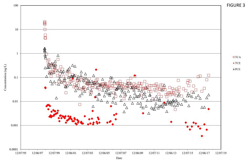
PRIMARY CHLORINATED VOCs IN THE MRDS SVE EXHAUST (LOG SCALE)
