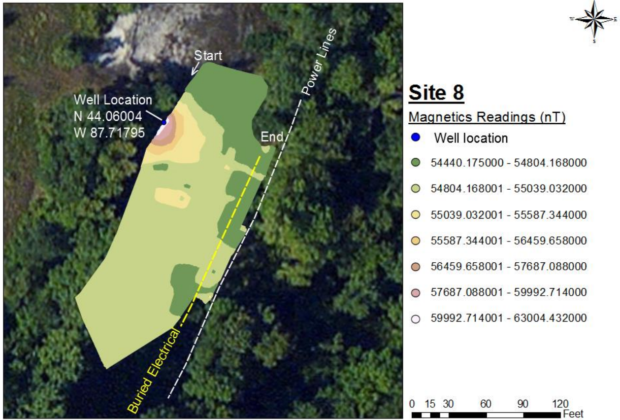
Figure 6. Survey Site 8 consisted of 18 lines starting to the northwest. Edge coordinates were not collected. The GPS coordinates recorded by the magnetometer were used for location.
