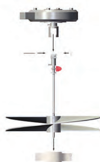
Impeller Assembly Removal Motion
