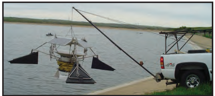
Hoisting SolarBee Out Of Water
