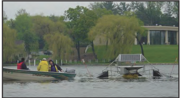
Towing SolarBee Using Small Boat
