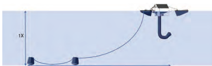
Mooring Block System (7:1 Scope)
