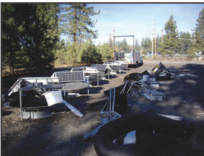
Staging Area With Disassembled SolarBee Units
