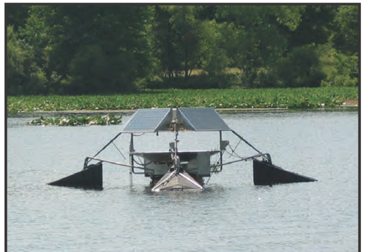
SolarBee in Raised Position, Ready to Tow
