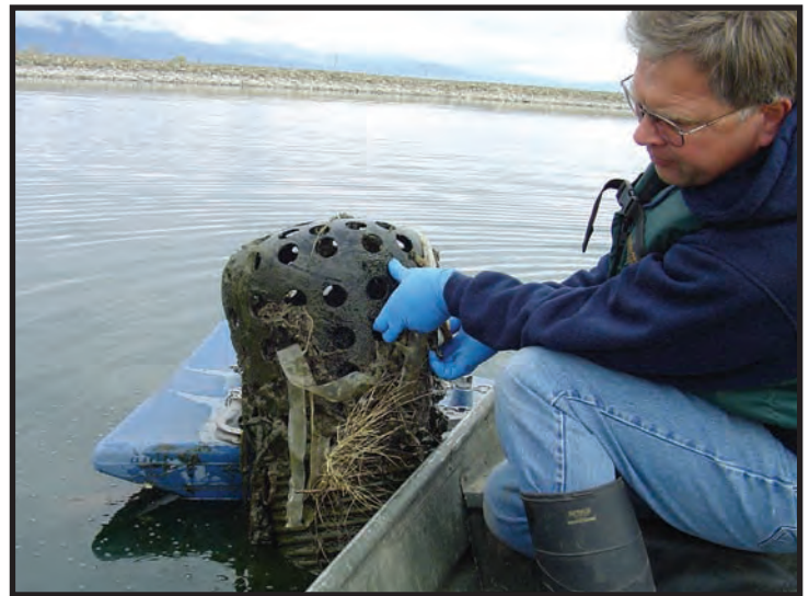
Partially Plugged Strainer
