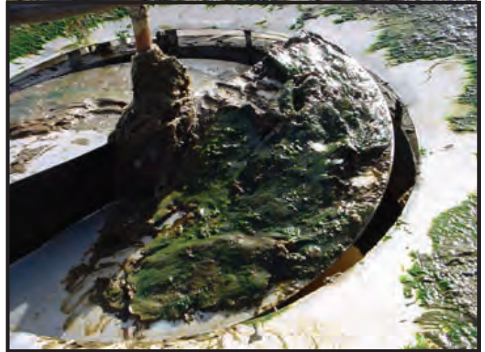
SolarBee With Buildup On Impeller
