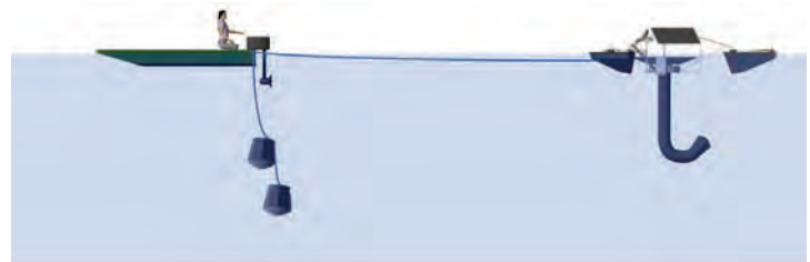
Mooring Blocks Suspended, Ready To Move
