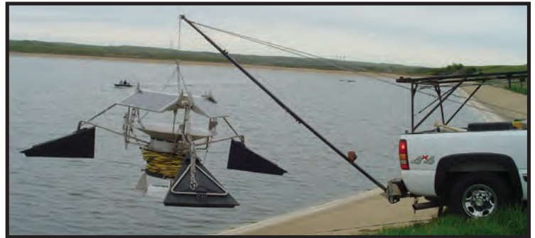
Hoisting SolarBee Out Of Water
