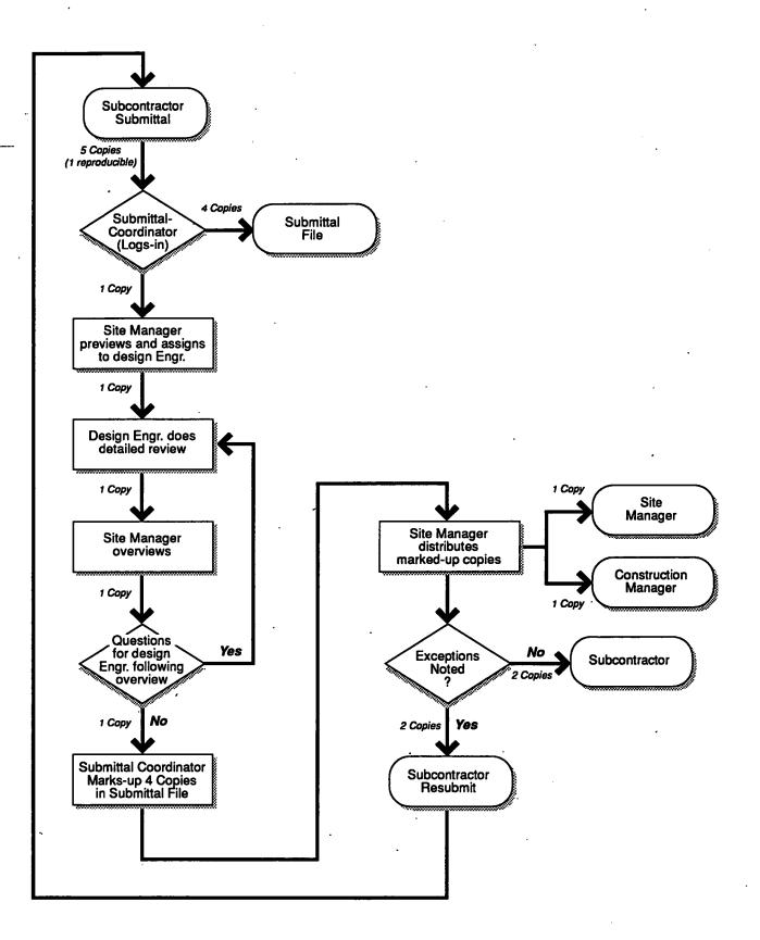
FIGURE 3-1 SUBMITTAL PROCESS FLOW CHART ONALASKA MUNICIPAL LANDFILL SITE LANDFILL CAP REMEDIAL ACTION
