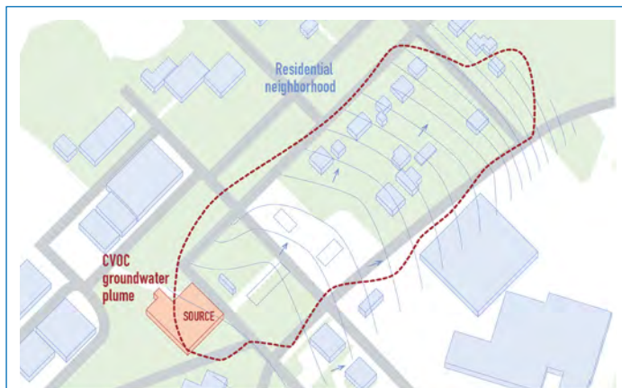
The extent of the groundwater CVOC plume circa 2010. The plume moved south to north through a residential neighborhood toward the Paw Paw River to the north.
