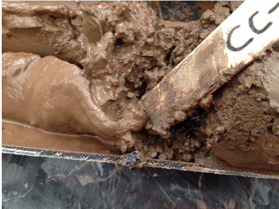
Sample (CC-023-A)- with Chunks of coal tar like material, NAPL, Stains and Sheens
