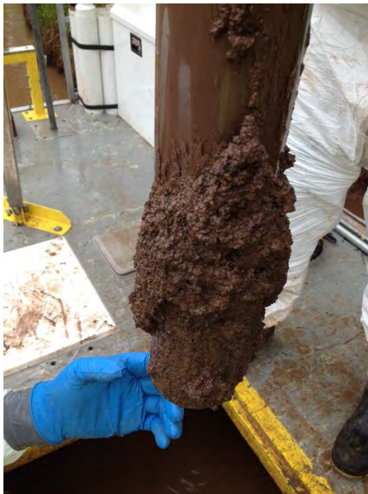
Core Sample collected in Crawford Creek with Creosote Impacts, Staining, Odors and Sheen
