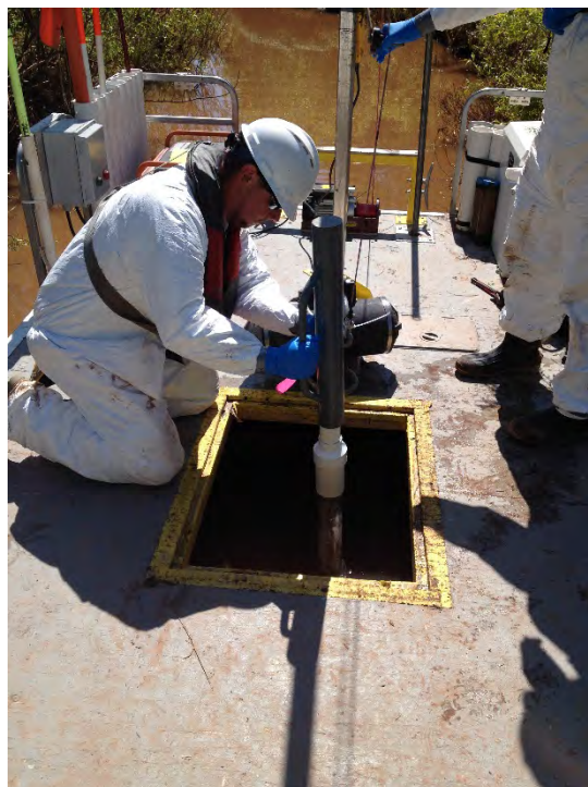
Typical Manual Coring setup from vessel
