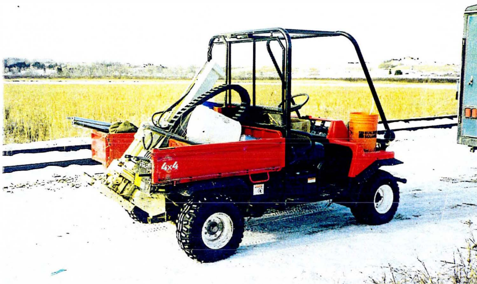
Photo 4: Four-Wheel Drive Mounted Hydraulic Soil Probe
