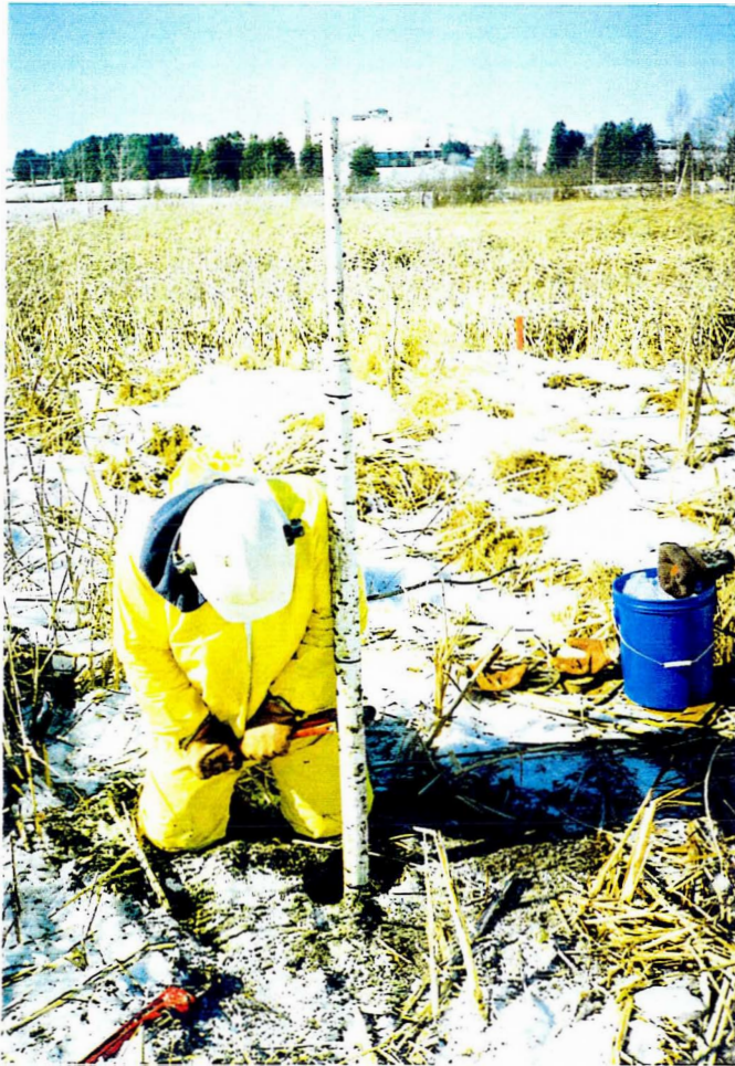
Photo 5: Modified Piston Sampling Technique
