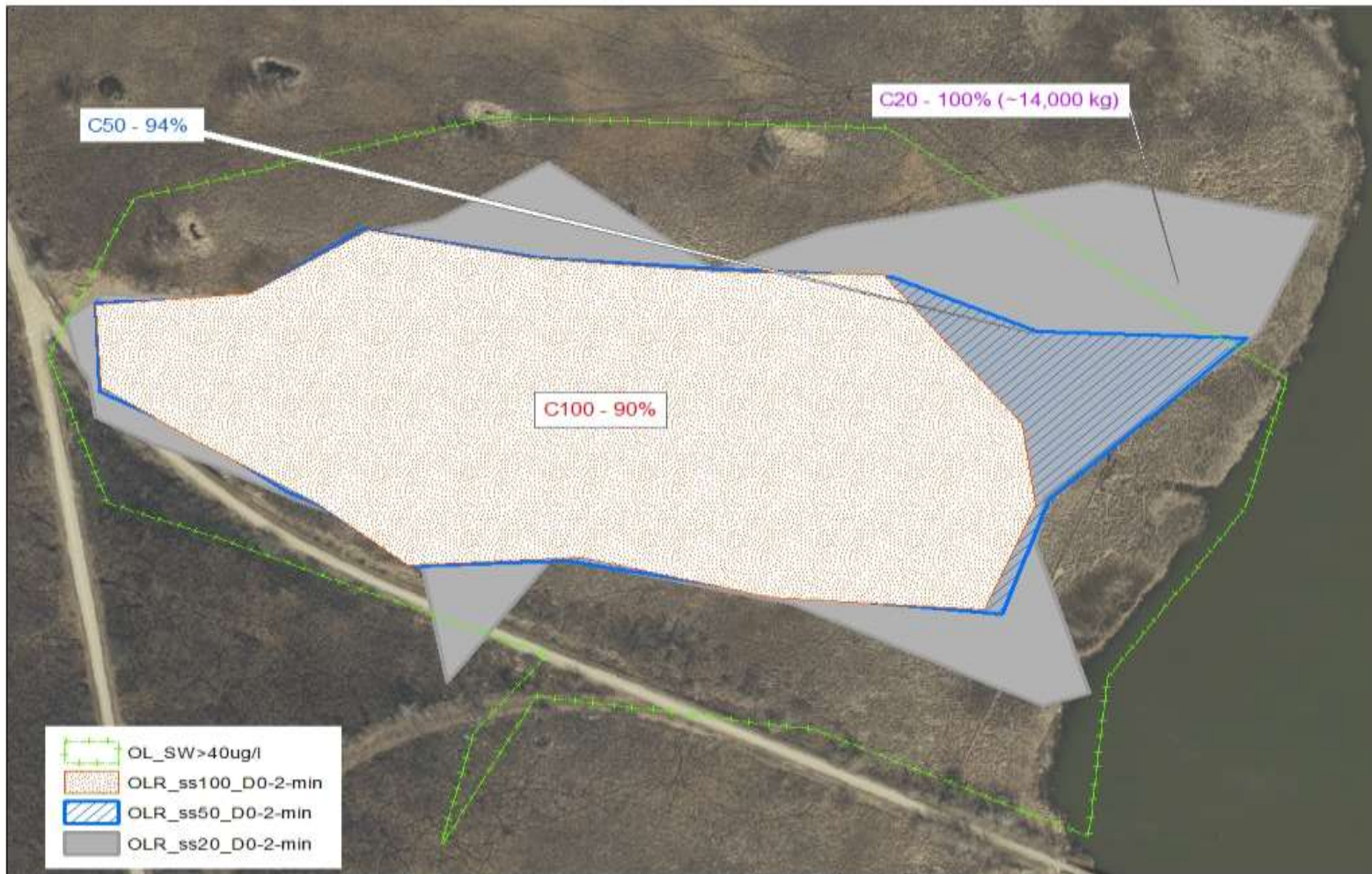
Fig. 14 Comparison of minimum extent and arsenic mass in percent for SS segment interval of 0-2 ft under scenarios C50 and C100 to maximums under C20 (Legend example: OLR_sed100_D0-2min: outline of arsenic concentration \geq 100 mg/kg in SS for depth 0-2 ft based on core samples as minimum extent; C50 – 94% and C100-90%: mass under C50 and C100 relative to that under C20 ; C20 -100%(~14,000kg): total mass under C20 in layer 0-2ft; OL_SW>40 ug/l: a reference for comparison to the extent of concentration at 40 ug/l in SW)
