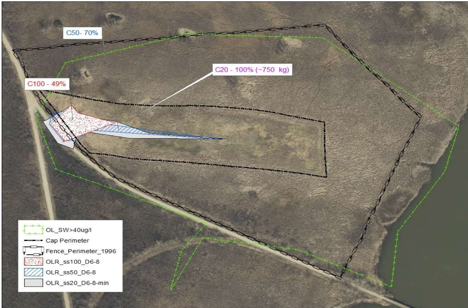
Fig. 19 Comparison of extent and arsenic mass in percent for SS segment interval of 6-8 ft under scenarios C50 and C100 relative to the minimums under C20 (the legend and labels are similar to Fig. 16 except for the segment interval and minimal value for C20 .)
