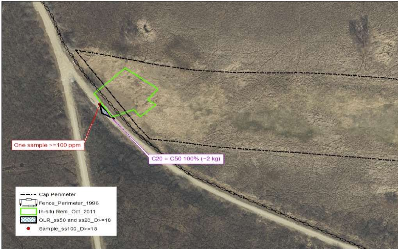
Fig. 25 Comparison of extent and arsenic mass in percent for SS deeper than 18 ft under scenarios C50 and C100 to the maximums under C20 (surface areas are the same for C20 and C50 . Only one sample exceeded 100 mg/kg)
