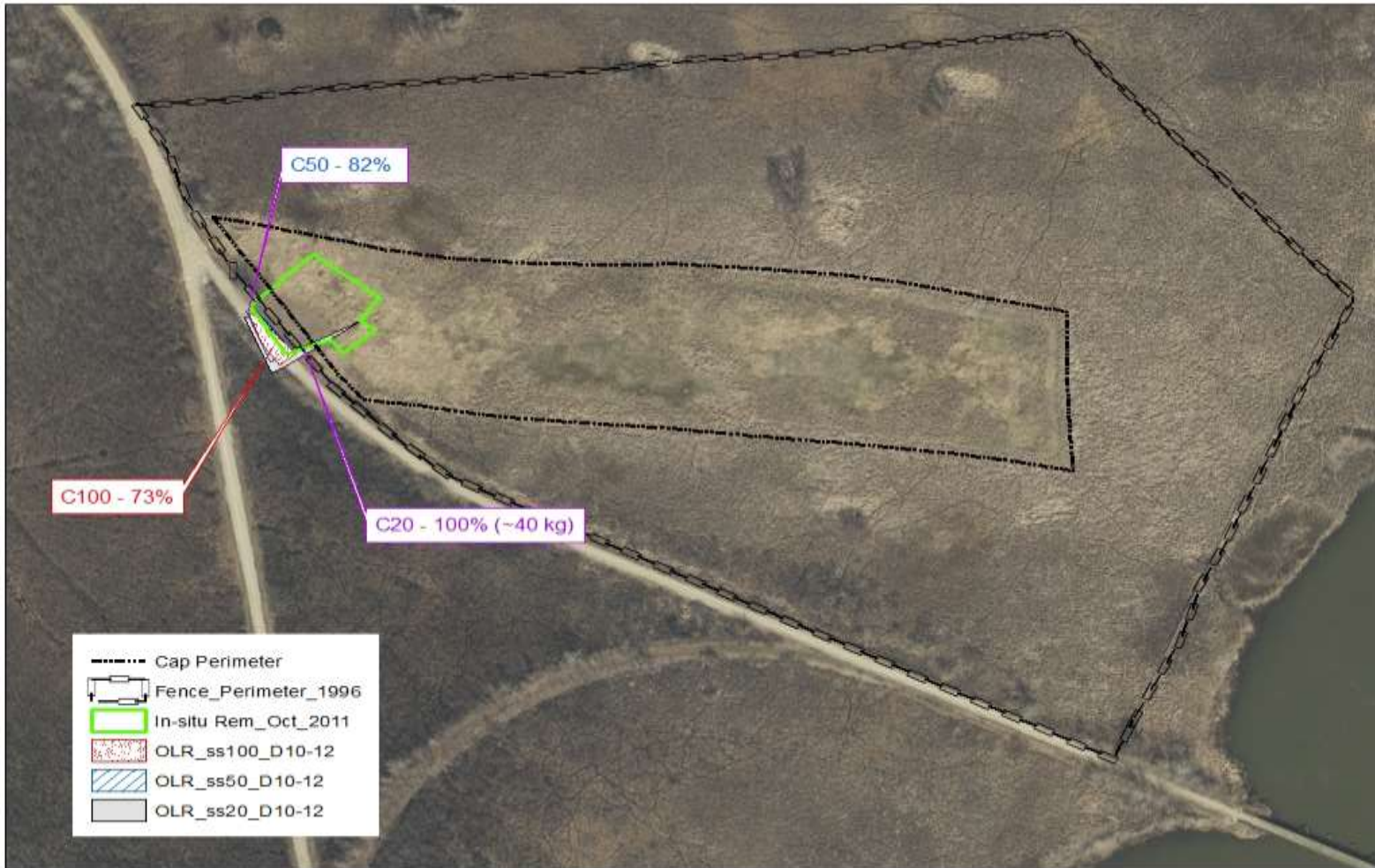
Fig. 23 Comparison of extent and arsenic mass in percent for SS segment interval of 10-12 ft under scenarios C50 and C100 relative to the maximums under C20
