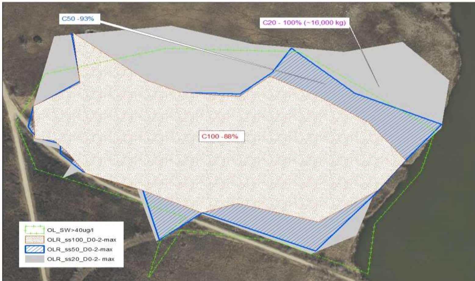
Fig. 15 Comparison of maximum extent and arsenic mass in percent for SS segment interval of 0-2 ft under scenarios C50 and C100 relative to the maximums under C20 (Legend example:OLR_sed100_D0-2max - outline of arsenic concentration \geq 100 mg/kg in SS for depth 0-2 ft based on combination of grab and core samples; C50 – 93% and C100-88%: mass under C50 and C100 relative to that under C20 ; C20 -100%(~16,000kg): total mass under C20 in layer 0-2ft; OL_SW>40 ug/l: a reference for comparison to the extent of concentration at 40 ug/l in SW)
