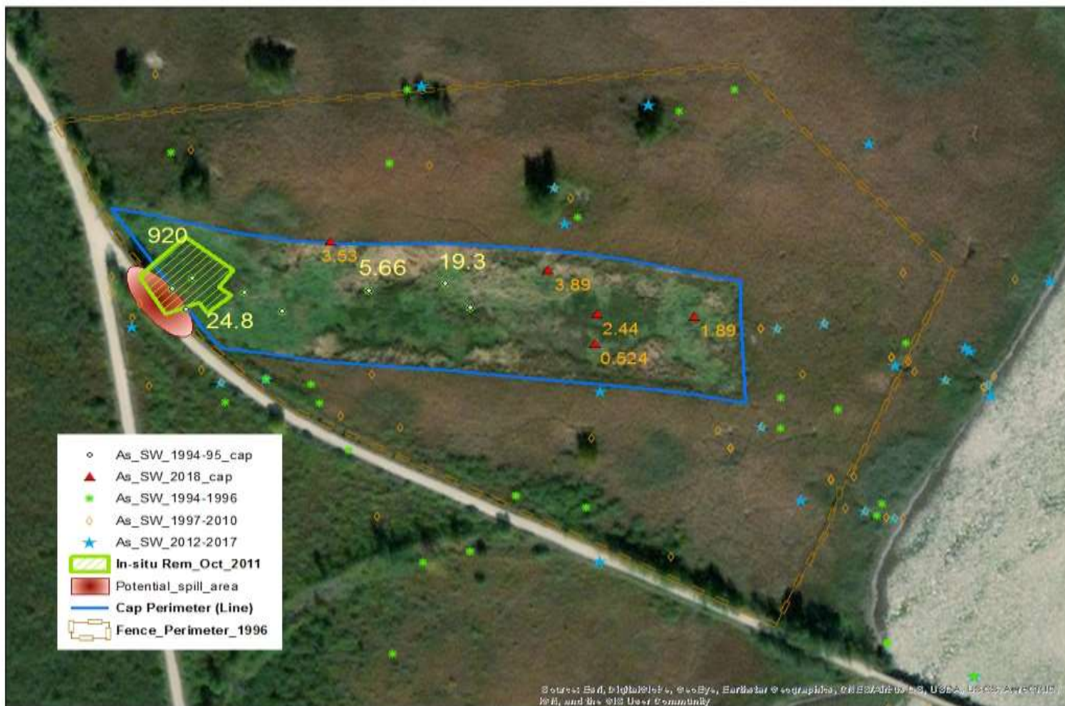
Fig. A-9 Spatial distribution of SW samples (1996-2018) with concentration labeled (mg/l) for samples collected from the capped area 1994-1995 and in 2018 (numerical numbers in yellow were for samples collected in 1994-1995 and in orange were samples collected in 2018)
