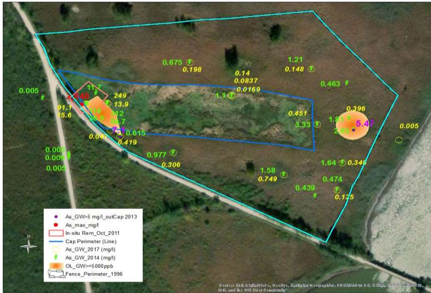
Fig. A-10 Spatial distribution of GW sampling wells with arsenic concentrations labeled for selected samples (As_GW_2014 and As_GW_2017: samples collected in 2014 and 2017 after in-situ remediation and the concentration are labeled in green and yellow, respectively. As_GW > 5 mg/l_outCap 2013: concentration detected > 5 mg/l and located outside of capped area are labeled in purple. As_max_mg/l: maximum arsenic concentration labeled in red.)
