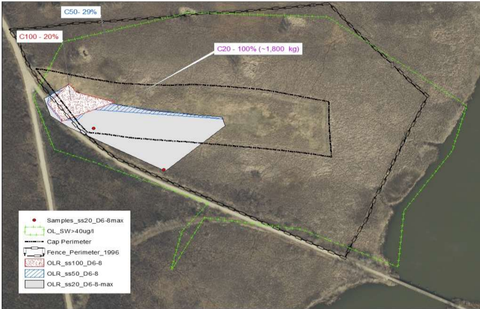
Fig. 20 Comparison of extent and arsenic mass in percent for SS segment interval of 6-8 ft under scenarios C50 and C100 relative to the maximums under C20 (the legend and labels are the same for Fig. 19 except for the segment interval and maximum extent for interval 6-8ft.)
