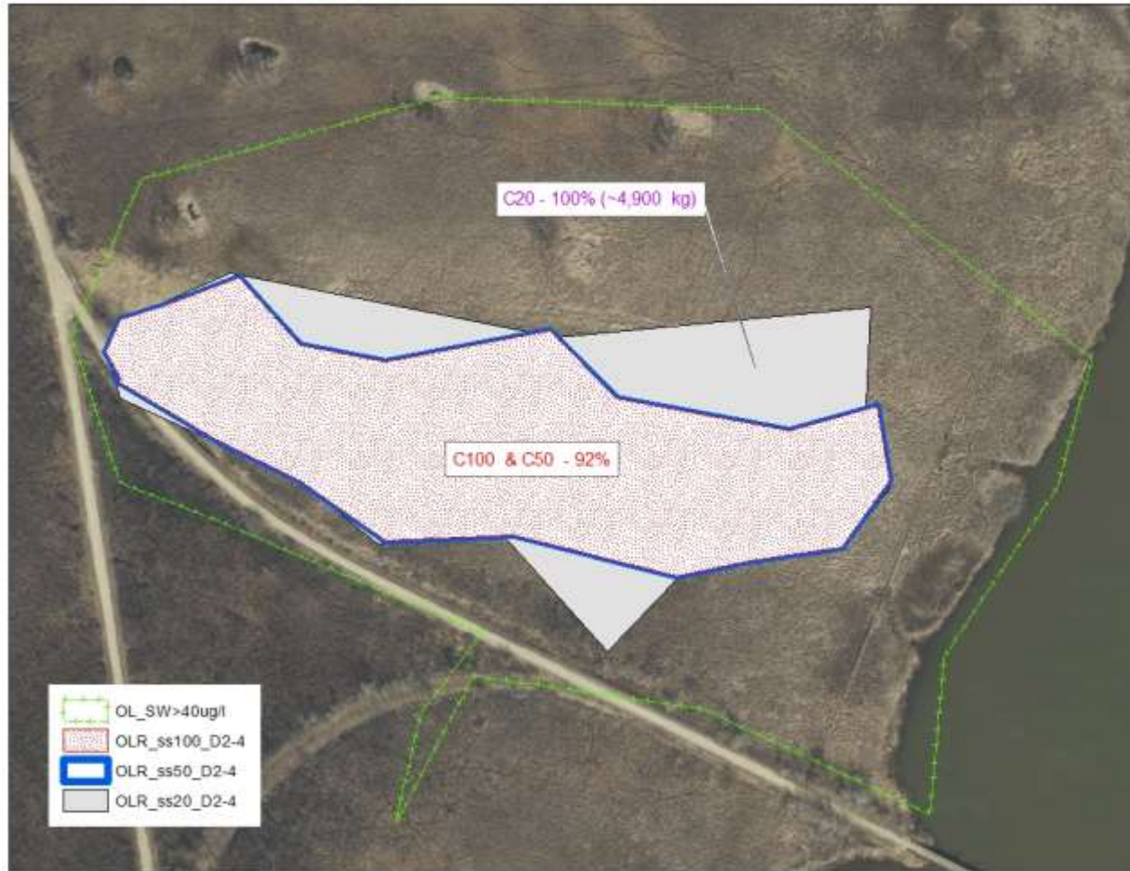
Fig. 16 Comparison of extent and arsenic mass in percent for SS segment interval of 2-4 ft under scenarios C50 and C100 relative to C20 (Legend example:OLR_sed100_D2-4 - outline of arsenic concentration \geq 100 mg/kg in SS for depth 2-4 ft based core samples; The horizontal extent for C100 is the same as that for C50 and so is the relative mass of 91%.); C20 -100%(~4,500kg): total mass under C20 in layer 2-4ft; OL_SW>40 ug/l: a reference for comparison to the extent of concentration at 40 ug/l in SW).
