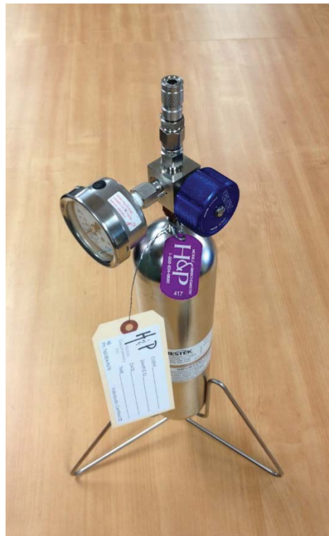
Photograph 10 – One-liter sampling canister with quick connect fitting (See Photograph 13, Item [A])
