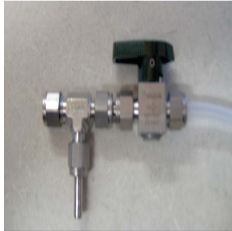
Photograph 17 - T-connection for quantitative tracer gas
