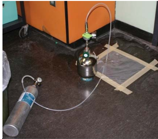
Photograph 21 - Plastic wrap leak detection method during sampling
