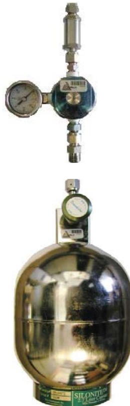
Photograph 12 - Flow Controller and Sampling Canister Flow controller (top) with inlet at top and outlet at base. Sampling Canister (bottom) with inlet at top. Note inverted nut at inlet of canister which threads onto flow controller outlet.
