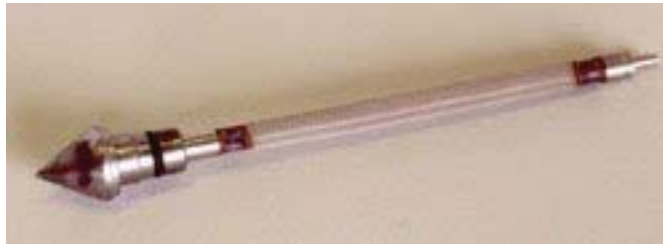
Photograph 7 – Stainless-steel mesh soil vapor point
