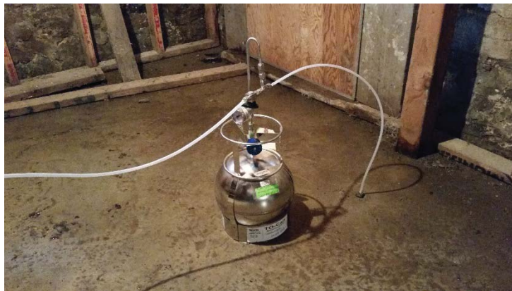
Photograph 6 – Sample collection at temporary sub-slab vapor point
