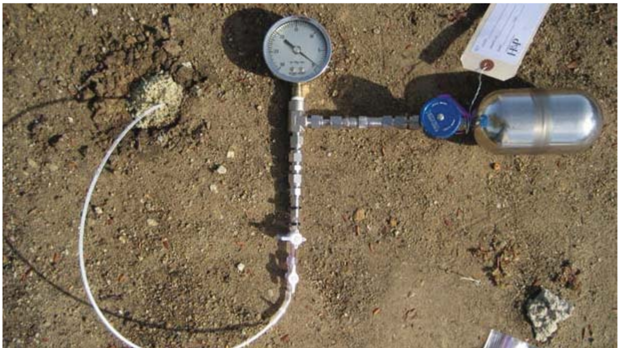
Photograph 8 – Soil gas sampling set up at deep, exterior temporary soil vapor point
