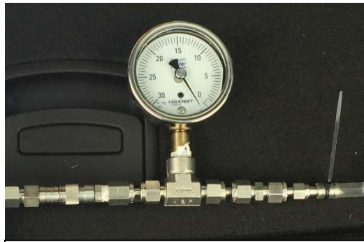
Photograph 11 – Flow controller with quick connect fitting to canister and barbed fitting to vapor point (See Photograph 13, Item [B])
