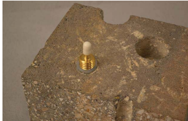
Figure 3. Installed VAPOR PIN®
