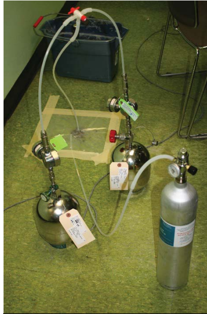
Photograph 15 - Field duplicate sample collection setup
