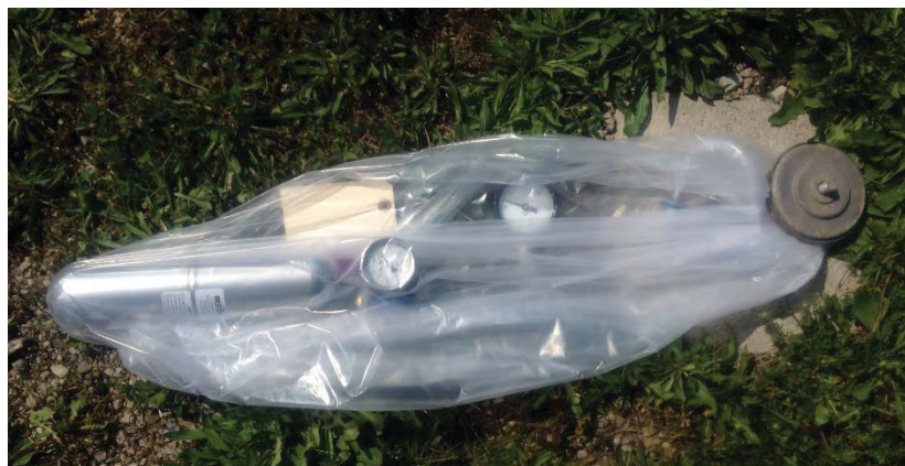
Photograph 20 – Soil gas sample collection set up at deep soil gas vapor point with shroud to contain 1,1-difluoroethane tracer during sample collection.
