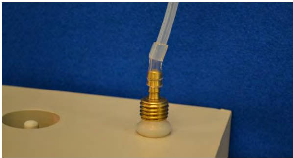
Figure 5. VAPOR PIN® sample connection
