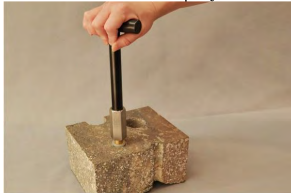
Figure 7. Removing the VAPOR PIN®
