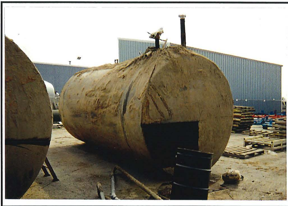
The Hydraulic Oil UST after removal.
