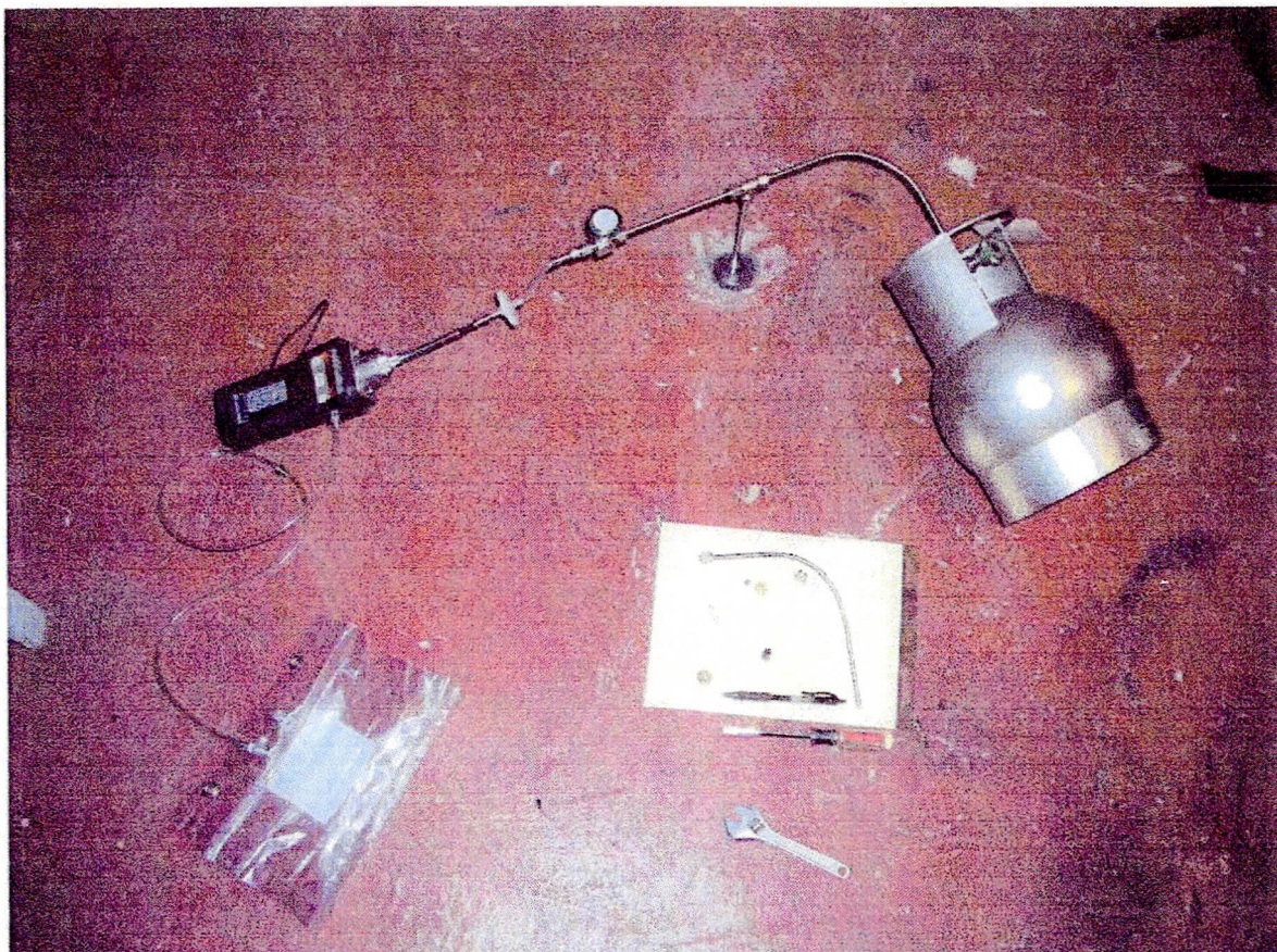
Figure 3: Sampling of sub-slab soil vapors, sample Port B, West Allis home, April 2006.
