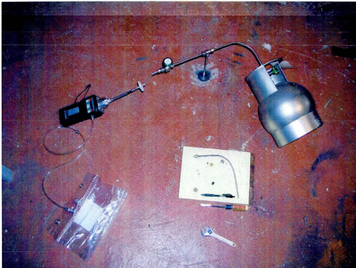
Figure 4: Sampling of sub-slab soil vapors, Sample Port B, West Allis home, April 2006.
