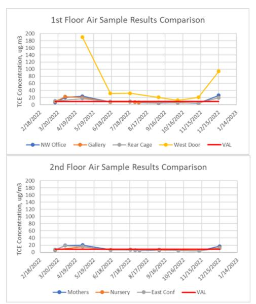
The TCE concentrations in the basement air samples are consistently only slightly greater than the 1<sup>st</sup> and 2<sup>nd</sup> floors, except for the West Stair Exit Door. The basement concentrations may be affected by the connection of the stairwell by the West Stair Exit Door to basement. The concentrations in the basement are significantly less than the West Stair Exit Door sample indicating that the concentration may be a result of indoor air mixing.
