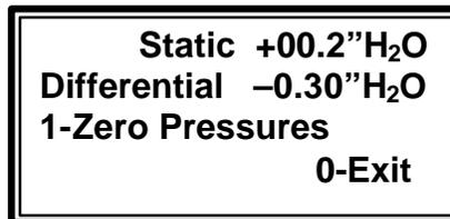
**Note: Units displayed are inches of water column or (millibar) MB depending on measurement unit selected (USA or metric).**
