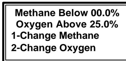
**NOTE:** To turn off alarms, set methane alarm to 00.0% and oxygen alarm to 25.0%.
