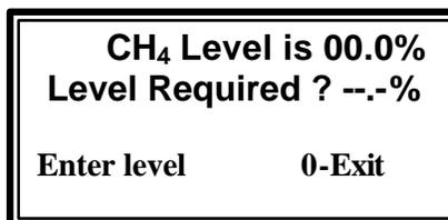
**Note:** If the GEM-500<sup>Ω</sup> receives CH<sub>4</sub> at or below this set point during the Read Gas Levels procedure, an audible alarm sounds to alert the operator.
