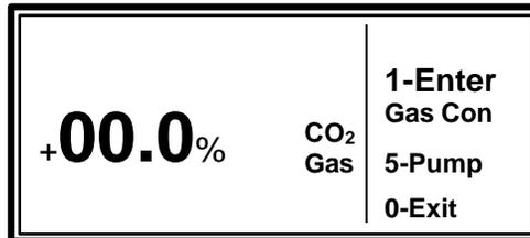
4. Press the **1** KEY, **Enter Gas Con**, to access the Enter Concentration screen (Figure 3.18). Input the percentage of Carbon Dioxide concentration of the calibration gas as three digits XX.X%. (40% Carbon Dioxide would be input as 400) The GEM-500™ will automatically place a decimal point in the proper position. After the percentage is entered, press the **0** KEY, **Exit**.
