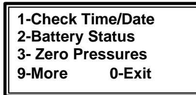
3. Figure 4.15 displays the current readings of the static and differential pressure transducers. If both pressures do not read 00.0 **DISCONNECT ANY HOSES ATTACHED TO THE GEM-500™** and press **1** KEY, **Zero Pressures**.
