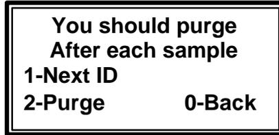
28. The Warning screen displays to remind the user to disconnect the hoses from the wellhead before starting the purge process. Once the hoses are removed, press the 1 KEY to begin the purge (Figure 5.50).
