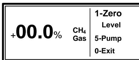
3. If using air to zero methane, press the **5** KEY, **Pump**, to turn on the GEM-500™ sample pump. Calibration gas hoses should not be attached to the GEM-500™ during this procedure. Allow the pump to run for two minutes or until gas reading stabilizes. If using oxygen calibration gas to zero methane, see step 3-6 in the Span Methane section then return to step 2 of this section.
