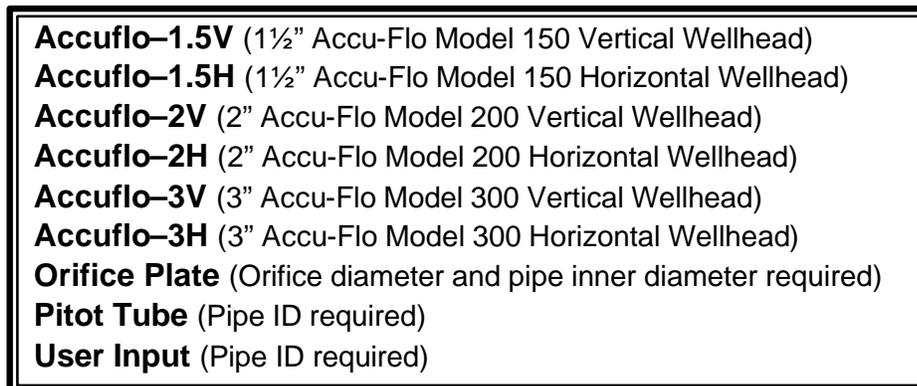
11. If an Orifice Plate, Pitot Tube or User Input flow device is selected, additional information is required. If the pipe or orifice diameter screen appears, input the required size as necessary. Insert inches or centimeters (depending on whether USA or Metric Units were selected on the General Utilities USA/Metric units screen). The unit uses XX.XX as the format and automatically enters the decimal point. Press the **0** KEY to enter and continue.
