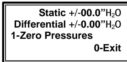
**Note:** The units displayed are in inches of water column or MB depending on whether USA or Metric was chosen in the General Utilities USA/Metric Units screen (page 30).
