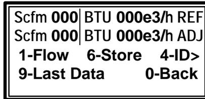
If the flow needs to be changed, adjust the control valve on the wellhead. Within a few seconds the new flow is displayed on the GEM-500™ as the adjusted value. When satisfied with the flow adjustment, press the **6** KEY to **Store** the information and continue to the Select Comments screen.
