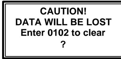
6. Enter 0102 from the keyboard and press the **0** KEY, Exit. The Clearing Memory screen displays for 3 seconds if the memory was erased.
