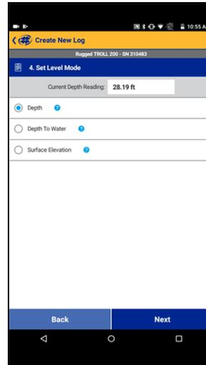
Select a level mode in step 4. Tap the blue circle to the right of each option for an explanation of how the mode works.
