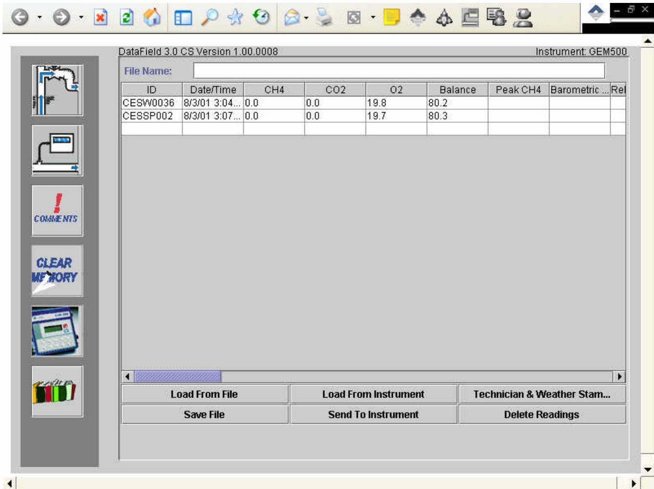
Once the file has been opened or data downloaded from the instrument, either **Save File** or **Send to Instrument** may be selected. If an attempt is made to save the data to an existing file, a warning message will display indicating the file will be overwritten and data lost. Data sent to the instrument will be displayed as the previous sampled readings for the selected ID.
