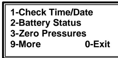
3. The gas calibration function is not on the first General Utilities screen. To reach this screen, press **9** KEY for **More** and **6** KEY for **Gas Calibration** (Figure 3.4). You may also press the **6** KEY while at the first General Utilities Screen to proceed directly to the Gas Calibration screen.
