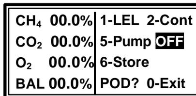
POD refers to interchangeable electrochemical gas pods that are used to extend the measurement capabilities of the GEM-500™ (Figure 5.8). These pods are available in seven different gases with nine different ranges and easily plug into the data port. The reminder lets the user know that if a pod were attached at this time, additional gas readings could be taken.
