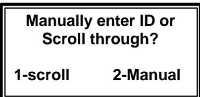
2. To scroll through the existing list of well ID's, press the **1** KEY, **Scroll**. The Select ID screen displays a single ID at a time. Use the **1** KEY (**UP ARROW**) or the **6** KEY (**DOWN ARROW**) to scroll through the list. When the ID of choice is displayed, press the **2** KEY, **Select**. (Figure 6.5)
