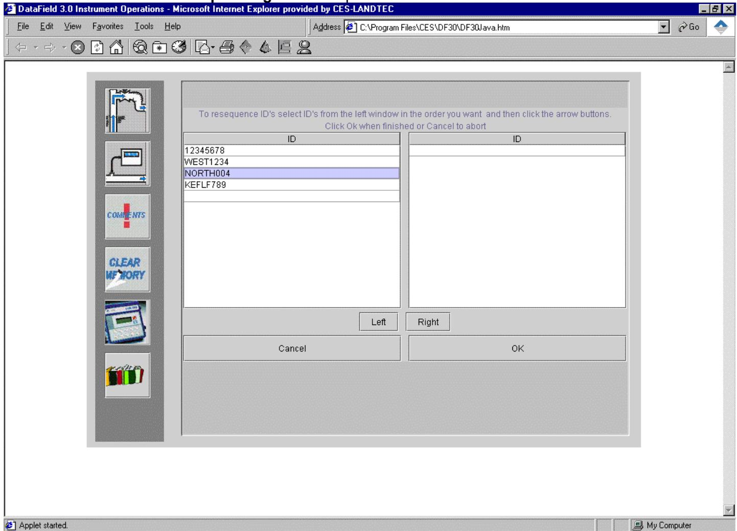
Select the ID from the left side window and click on the **Right** button to move ID to the right window to create the new sequence order. Repeat this process moving all ID's to the right side of the desired order.
