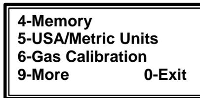
4. Pressing the **6** KEY for **Gas Calibration** on the General Utilities Sub-Menu screen, the first Gas Calibration screen is displayed as shown in Figure 3.5.
