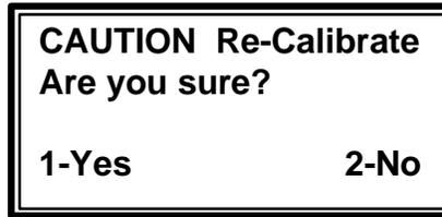
6. Press the **1** KEY, **Yes**, and one of the two following messages will appear (Figure 3.20 or Figure 3.21). If the Calibration OK screen appears, go to step 9 below.
