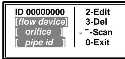
11. To edit the chosen Well ID information, press the **2** KEY, **Edit**. Use the **1** KEY (**UP ARROW**) or the **6** KEY (**DOWN ARROW**) to scroll through the choices listed in Figure 4.33. Once the desired flow device is located in the shaded selection window, press **0** to select and **Continue**. Press the **0** KEY, **Exit**, to return to the ID Maintenance screen. (Figure 4,38)
