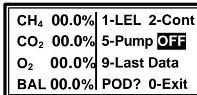
POD refers to interchangeable electrochemical gas pods that are used to extend the measurement capabilities of the GEM-500™ (Figure 5.32). These pods are available in seven different gases with nine different ranges and easily plug into the data port. The reminder lets the user know that if a pod were attached at this time, additional gas readings could be taken.
