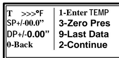
**Note: If flow measurement is required, temperature must be entered either manually or with the optional temperature probe.**
