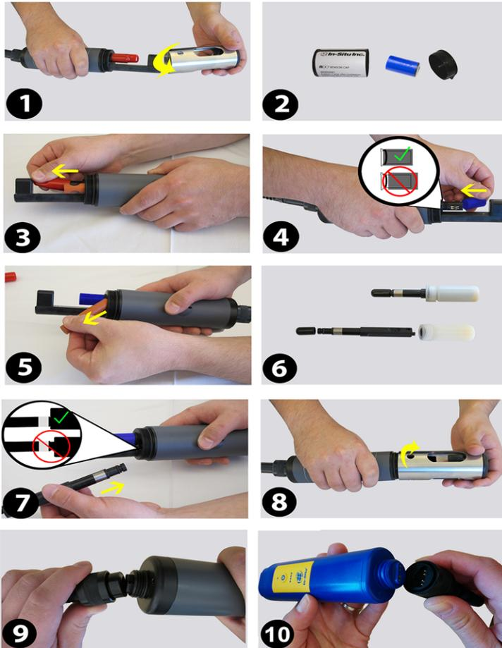
1. Twist the restrictor off the probe.
