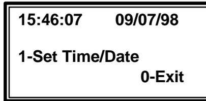
4. The time and date are displayed on the top line of the screen. A 24-hour clock or military time is used. If the time is after 12 noon, add 12 to the hour to convert it to the 24-hour format. Example: 3 p.m. is 12+3 = 15:00 hours. The time format is Hours: Minutes. Seconds. The date format used in the example is in U.S. calendar format with the month first and day second (mm/dd/yy).
