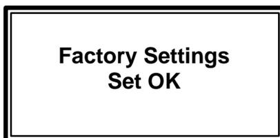
4. After loading the factory settings, the methane and oxygen calibration **MUST BE RE-ZEROED PRIOR TO USE**. After completing the gas calibrations, the GEM -500™ is ready to read gas levels. Go to Chapter 5 of this manual, Read Gas Levels.
