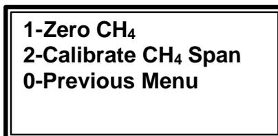
2. Pressing **1** KEY, **Zero CH<sub>4</sub>**, initializes the Zero Methane procedure (Figure 3.7). A methane percentage will not display until the Infrared (IR) Bench warms up. A plus or minus sign may appear on the far left of the display. This symbol may be ignored.
