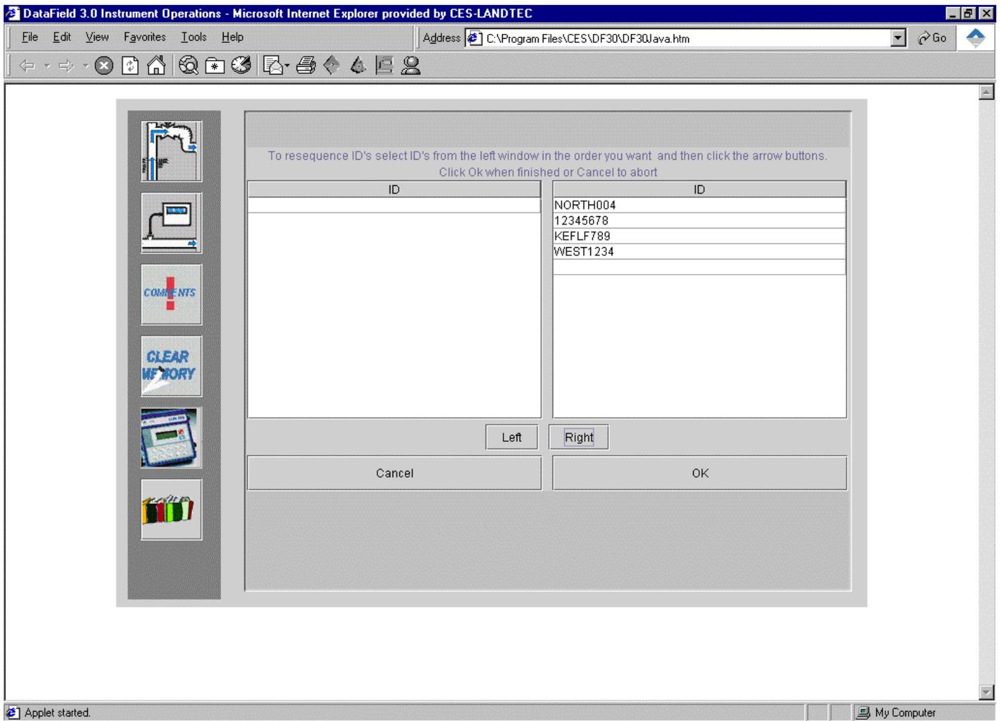
Click OK when the desired new sequence is obtained. Click on the **Save File** button to save the new data set to a file on disk or click on **Send to Instrument** to upload the new data to the instrument. Either action will overwrite the previous data.
