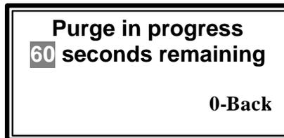
30. The pump will run for 60 seconds and then shut off allowing the next well ID to be displayed. (Figure 5.52)
