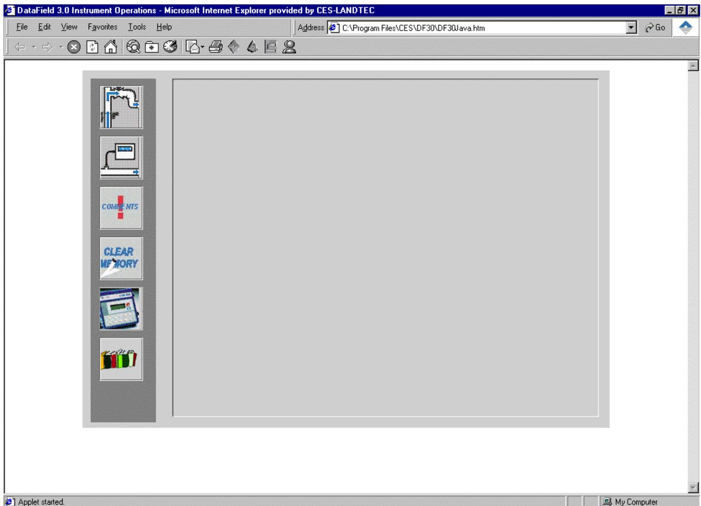
Six main categories (buttons) are listed down the left side of the screen: ID Functions, Download Comments, Clear Memory, Instrument Settings and Resource Links. Clicking on any one of the buttons will take the user to that functionality of the application.
