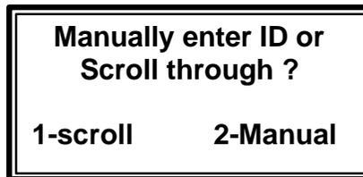
5. To scroll through the existing list of well ID's, press the **1** KEY, **scroll**. The Select ID screen displays a single ID at a time. (Figure 5.20) Use the **1** KEY (**UP ARROW**) or the **6** KEY (**DOWN ARROW**) to scroll through the list. When the ID of choice is displayed, press the **2** KEY, **Select**.
