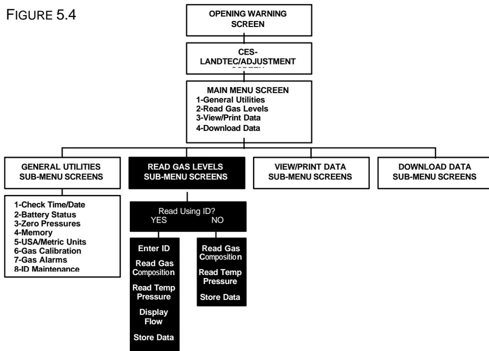
As shown in the screen tree diagram above (Figure 5.4), there are two menu paths that can be followed through the Read Gas Levels function. The path taken depends upon whether or not a well ID has been defined and stored in the GEM-500™. Well IDs can be added at several points during this procedure.
