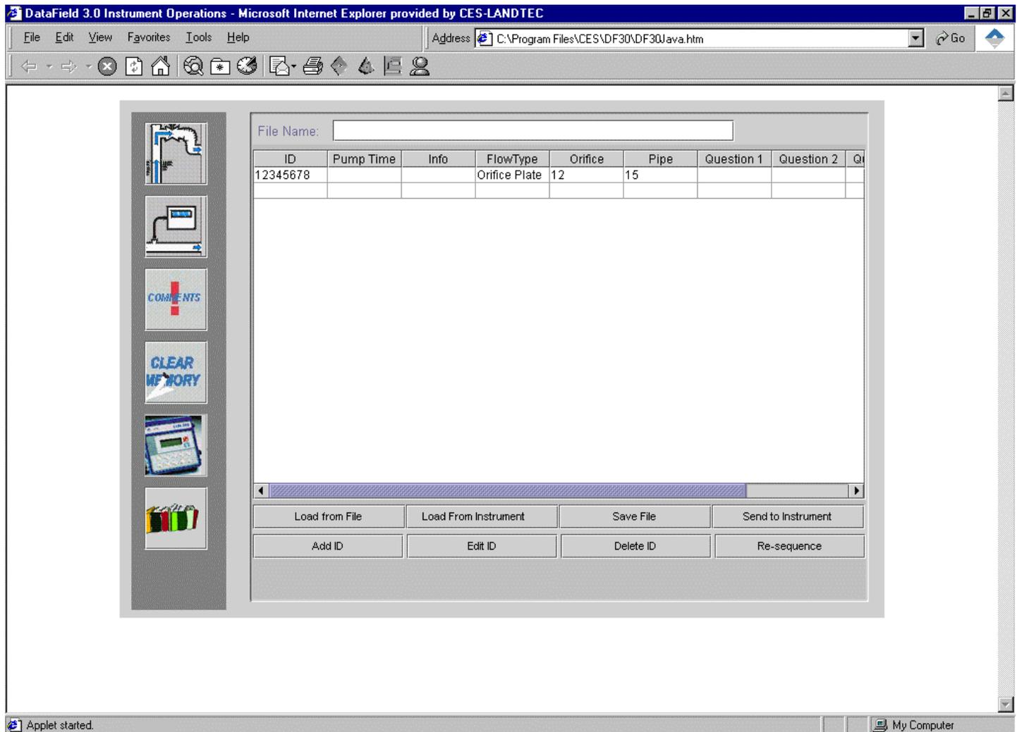
Once all the ID's have been entered, click **Save to File** button to save the ID data to a file or **Send to Instrument** button if data is to be uploaded to an instrument for field sampling.
