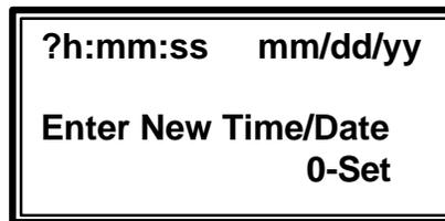
**NOTE:** If it is necessary to correct an entry error, use the **0** KEY as a **Backspace Key** by holding it down for 1 second. In normal use, the **0** KEY is quickly pressed and released.
