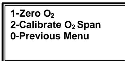
2. Press the 2 KEY, **Calibrate O<sub>2</sub> Span**, on the Oxygen Calibration screen will appear (Figure 3.28).
