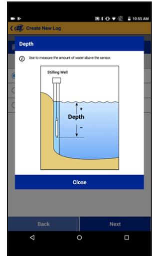
For Depth to Water and Surface Elevation modes, enter a level reference. See "About the Level Reference" on page 1 of this manual for complete information about level modes and level references.
