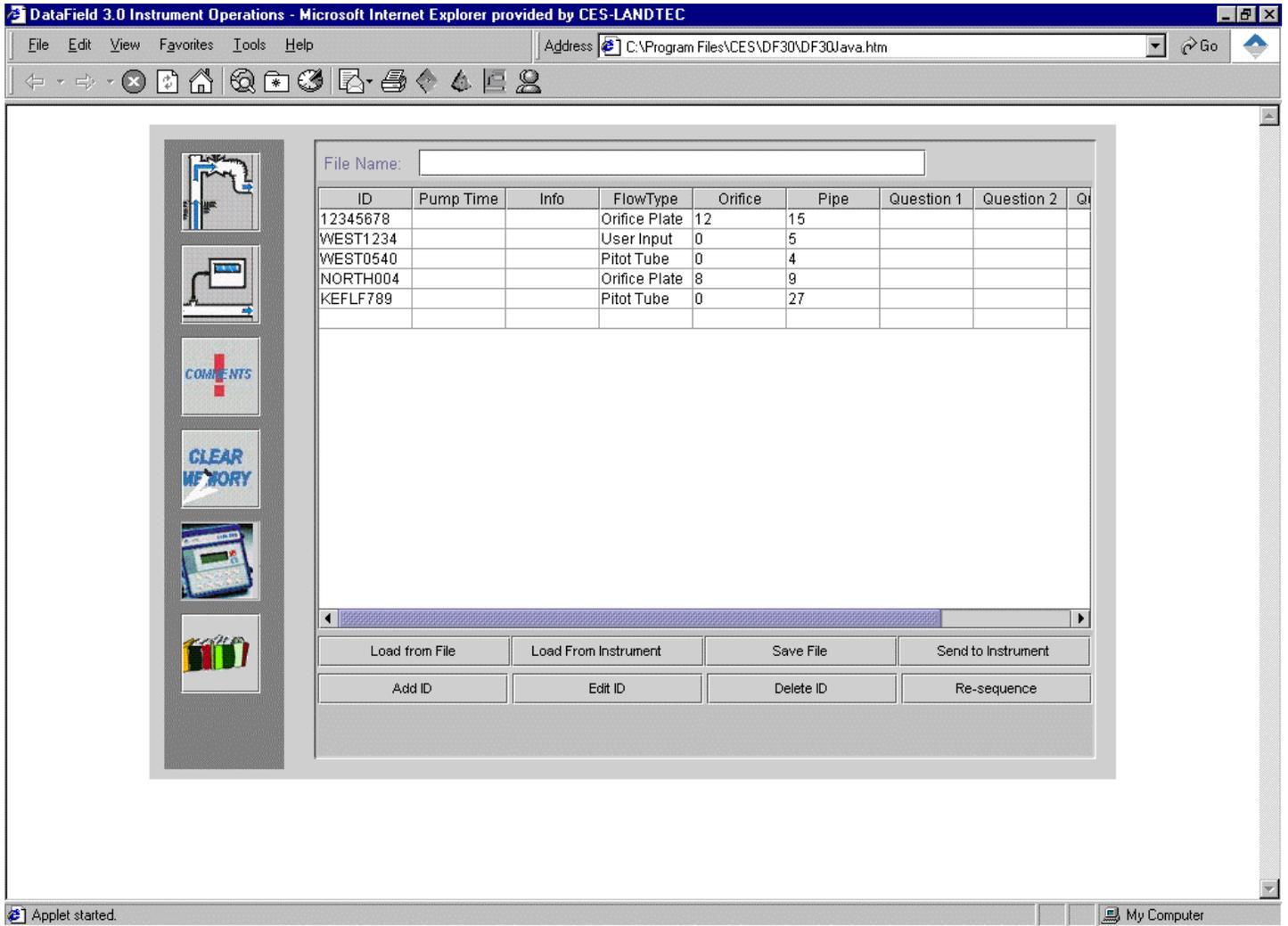
To select an ID for editing, click on the ID to highlight the ID, and then click on **Edit ID** at the bottom of the screen. The Edit ID screen will open and allow information for the selected ID to be changed. When finished with the changes, click on **Save** to save the edited ID to the ID list.
