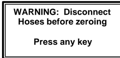
21. The pressures displayed on the Static/Differential screen are displayed with either a positive or negative and need to stabilize (quit changing) before being zeroed. When stabilized, press the **1** KEY to **Zero Pressures**. (Figure 5.39)
