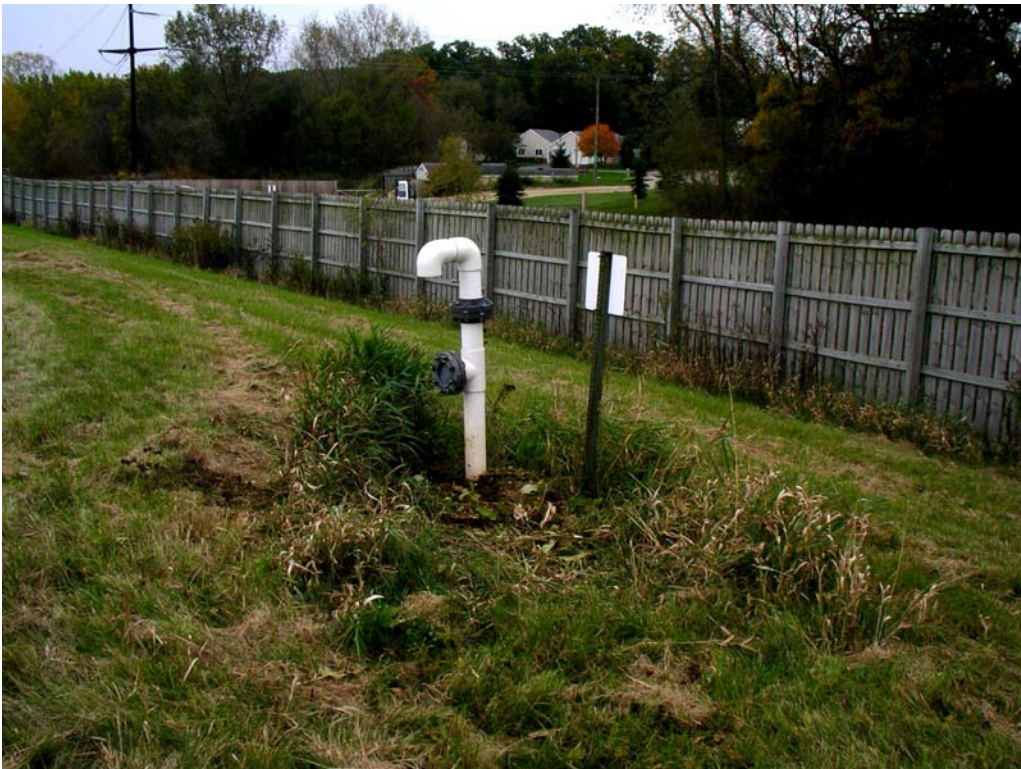
GV-11; viewed looking south. View following removal of deeper rooted woody vegetation.
