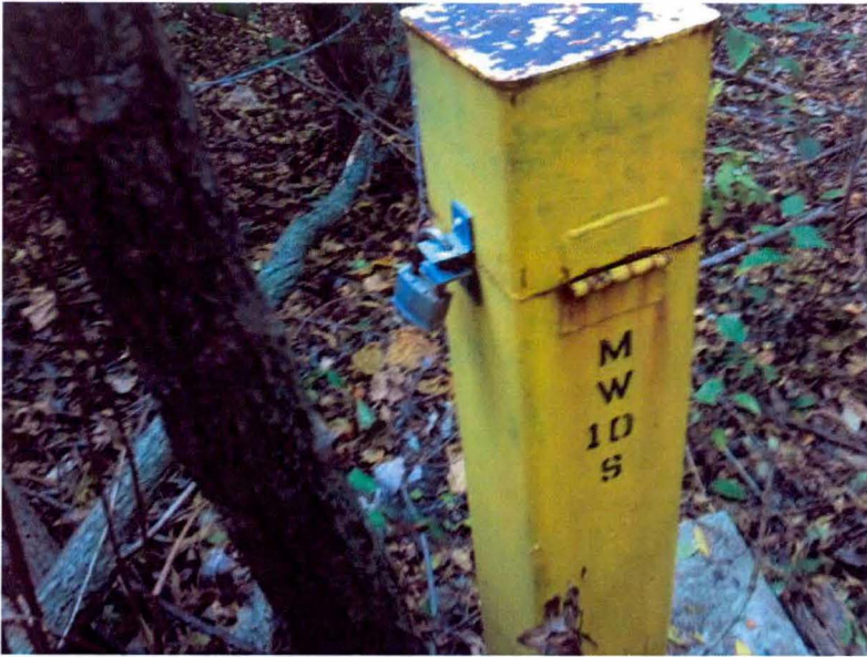
2012-09-09: Example of Lock Clasp for Securing Well Date: 01-Oct-2012 Time: 8:07 AM Weather: Sunny, 50 Degrees F.
