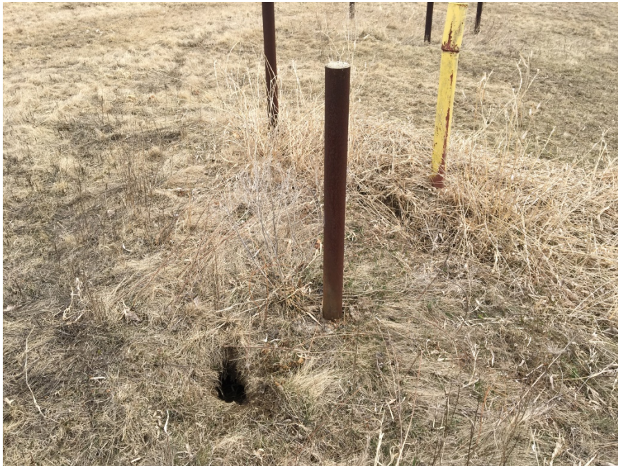
Photo 4: Animal burrow present near MW-2D (looking down).
