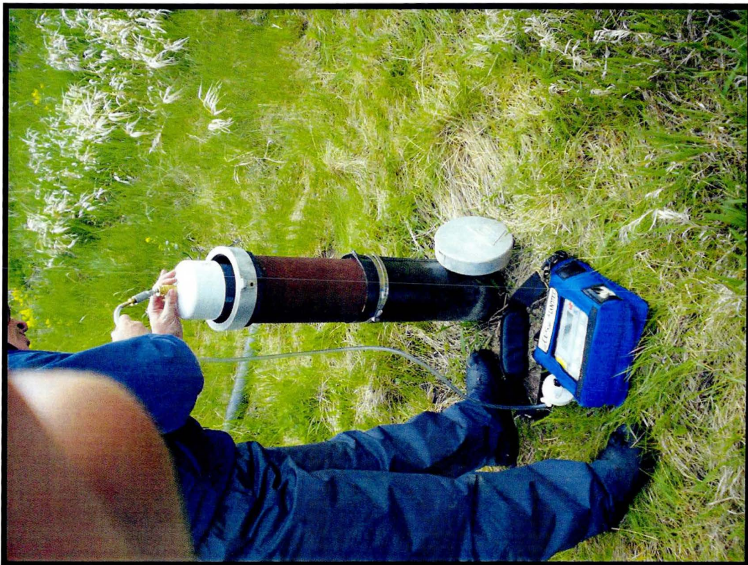
Taking gas measurements at leachate well LC-2
