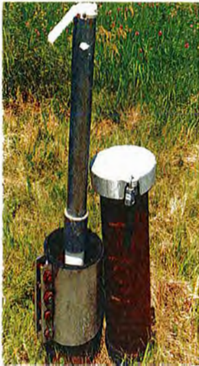
P-104, casing should be extended. It is damaging the well's discharge tubing.
