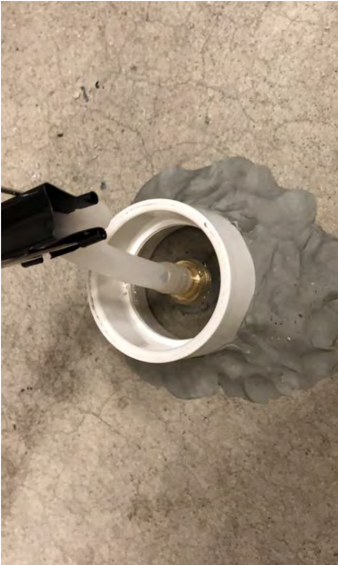
Photo 1: Water dam test at temporary vapor point VP-1
