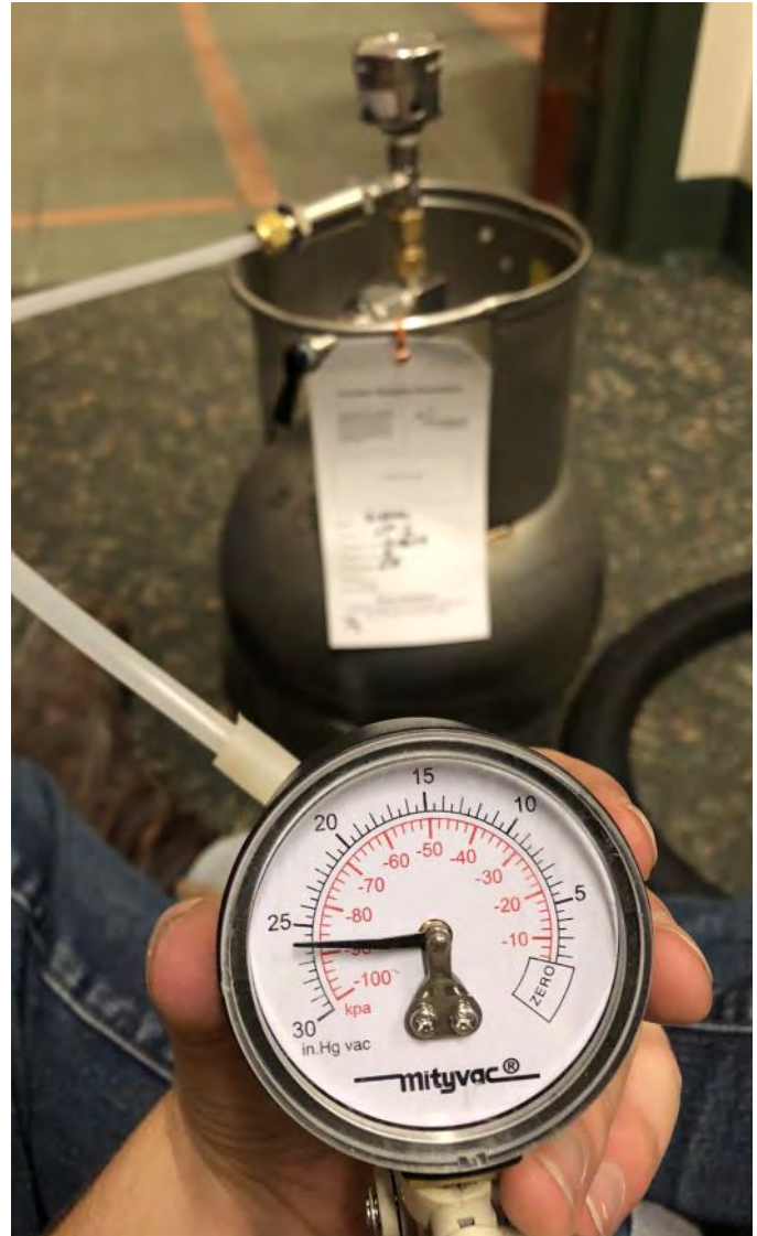
Photo 2: Shut-in test for temporary vapor point sample VP-6
