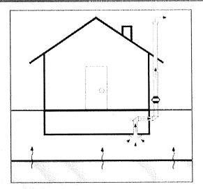
If potentially harmful chemical vapor intrusion is detected in a home or business, the most common solution is to install a sub-slab depressurization system. This system captures and redirects soil vapors from below the building foundation before they enter the indoor air. Vapors are vented outside of the building where they disperse into the air and are rendered harmless.
