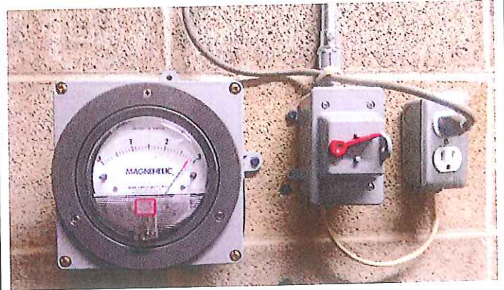
2. View of the Magnehelic pressure gage mounted behind the dry cleaning machine. The pressure gage is reading 2.5 inches of water.
