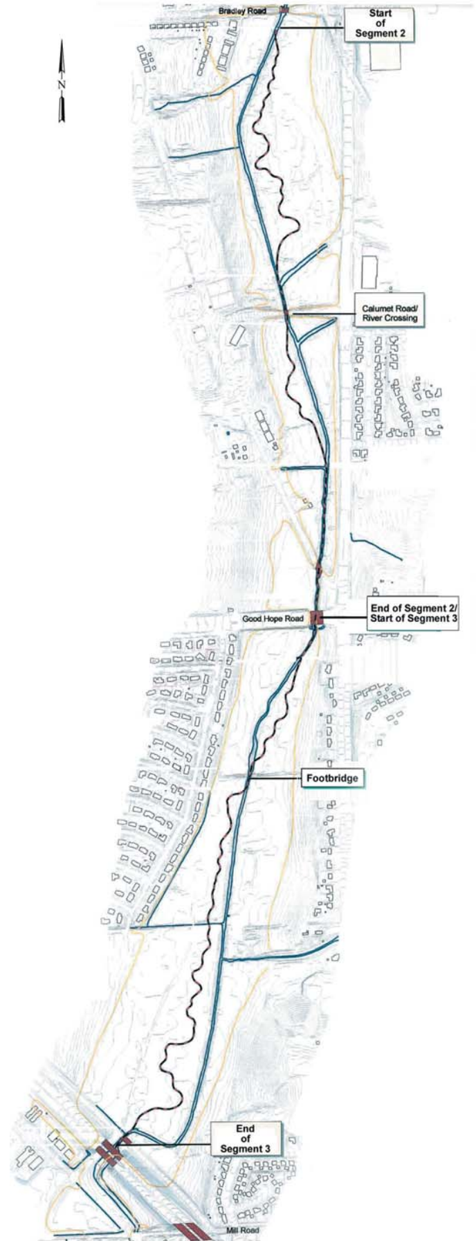
This map shows segments 2 and 3 of the Little Menomonee River. The straighter line represents the present channel. The wavy line represents the new sections.
