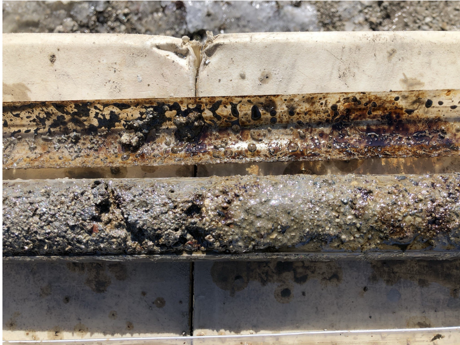
Photo 3: Soil boring GP-104, depth interval 10-15' bgs. Well graded brown, gray, red, and black sand with some gravel. Strong petroleum odor, dark staining, and free product from 12-13' bgs. Photograph taken on March 1, 2021.
