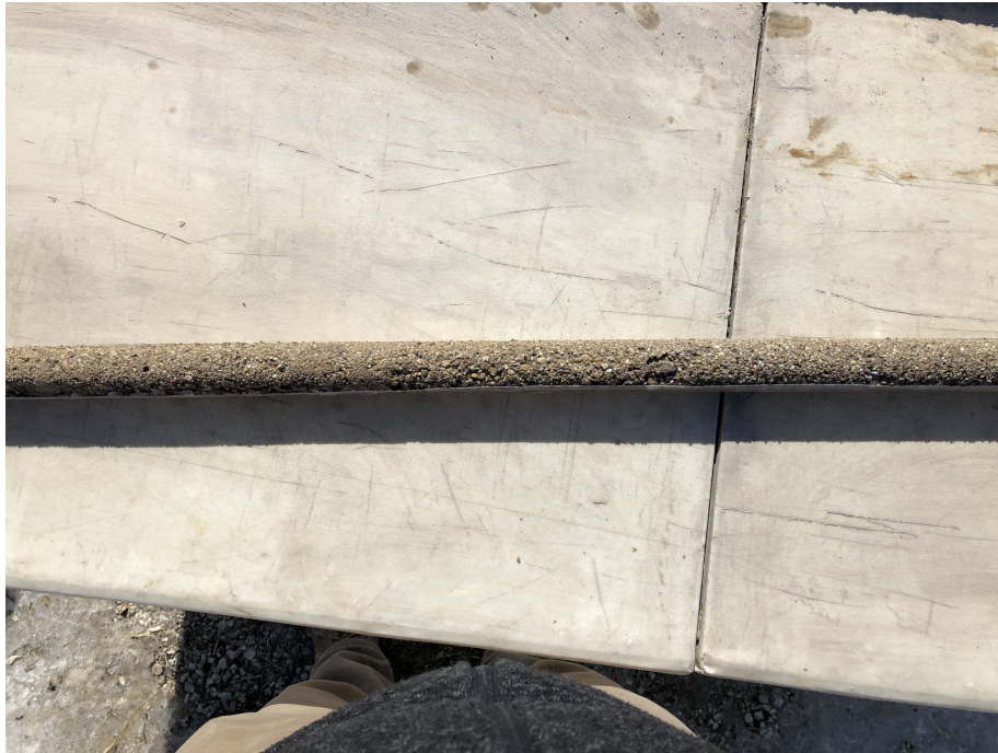
Photo 1: Soil boring GP-102, depth interval 5-10' bgs. Well graded brown, gray, red, and black sand with some gravel. Photograph taken on March 1, 2021.
