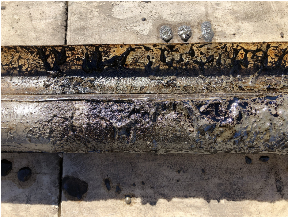
Photo 4: Soil boring GP-111, depth interval 5-10' bgs. Brownish gray, well graded clayey gravel. Strong petroleum odor, dark staining, and free product from 7.5-10' bgs.. Photograph taken on March 2, 2021.
