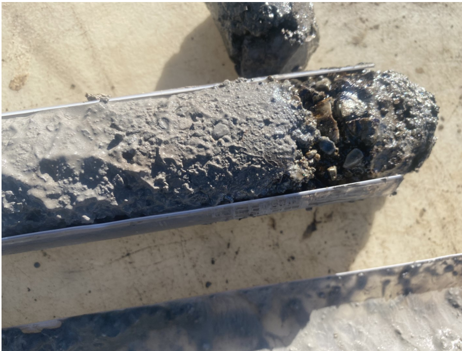
Photo 2: Soil boring GP-134, depth interval 5-10' bgs, close-up. Well graded gray, clayey gravel with some sand and trace free product. Photograph taken on January 20, 2022.
