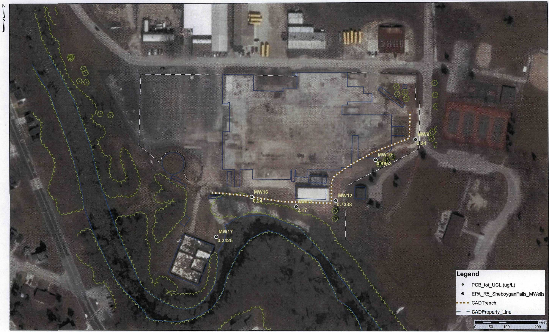
Figure 1 Sheboygan - Total PCBs in Groundwater (UCLs) Figure 7
