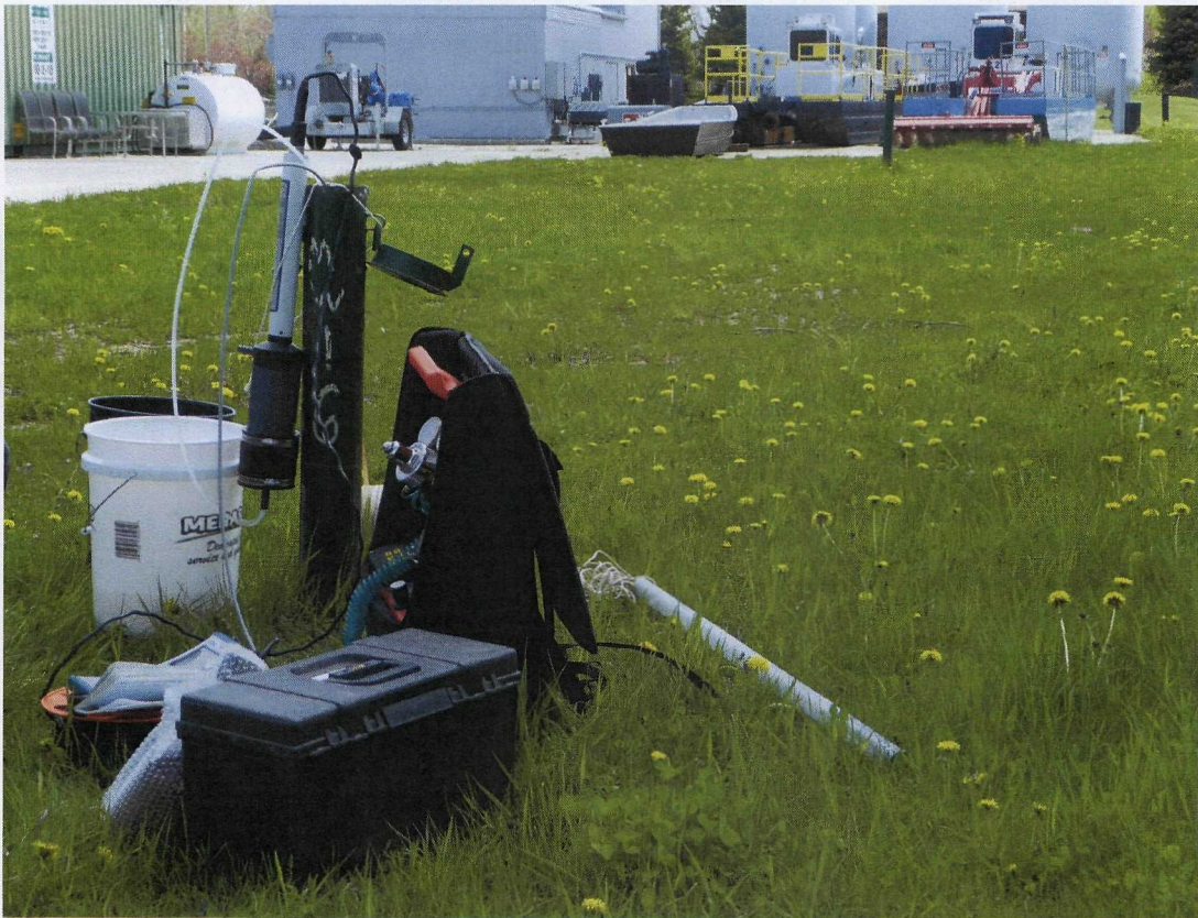
Monitoring well MW-16 being sampled at Groundwater Monitoring/ Interceptor Trench
