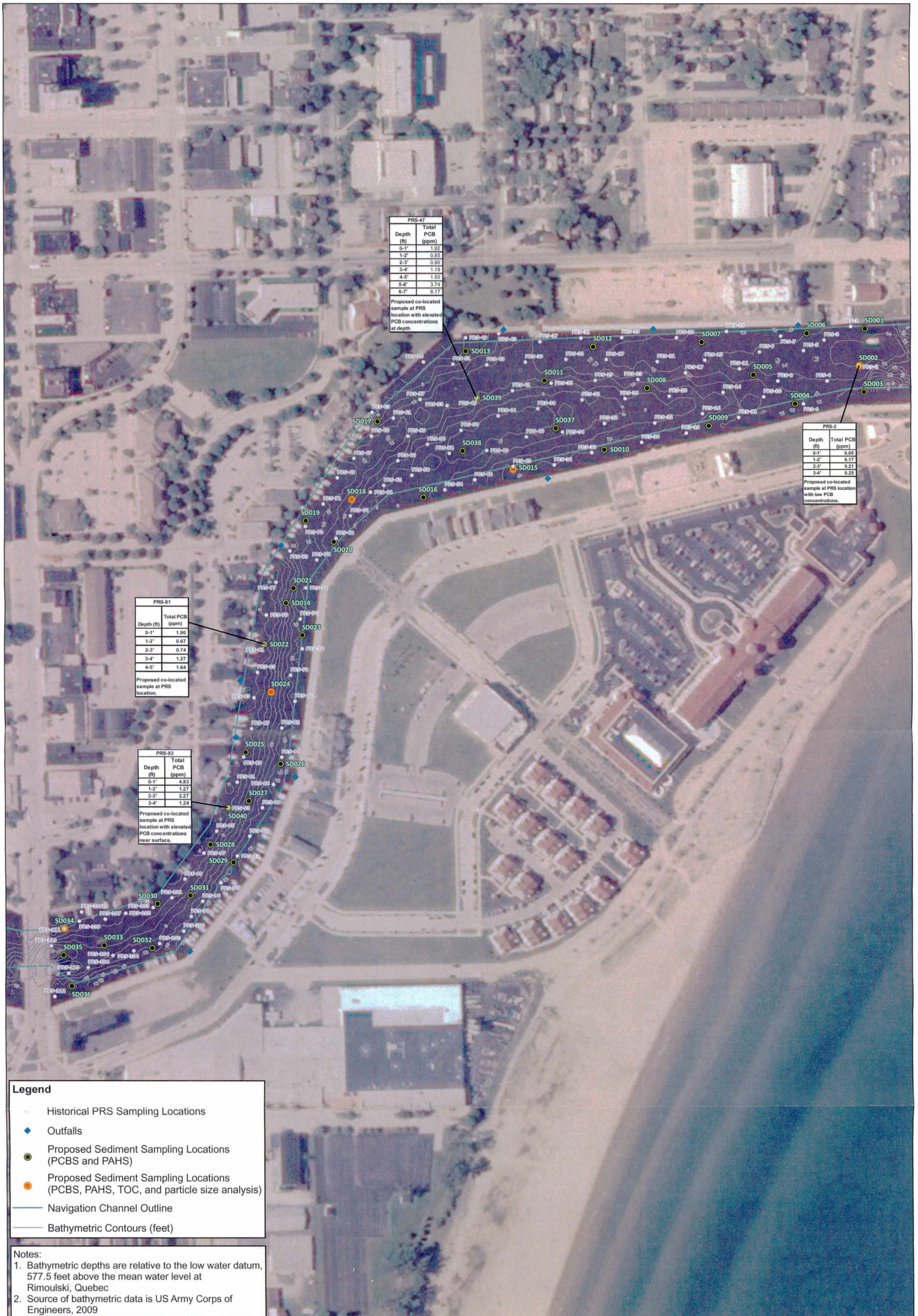
Figure 2 Proposed Sediment Sampling Locations Lower River and Inner Harbor of the Sheboygan River Remedial Investigation Sheboygan, WI
