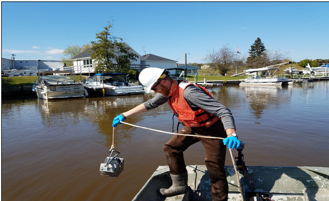
PHOTO NO. 8: View of sediment sampling method (typical Lower River and Inner Harbor).
