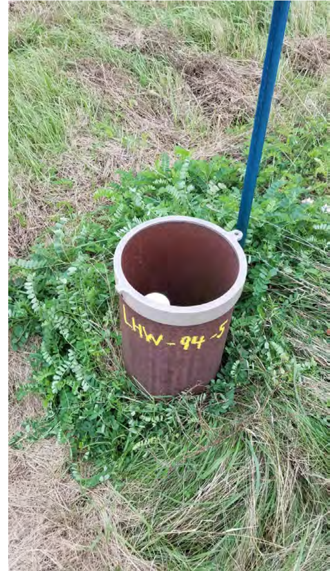
28. LHW-94-5 – no lock present
