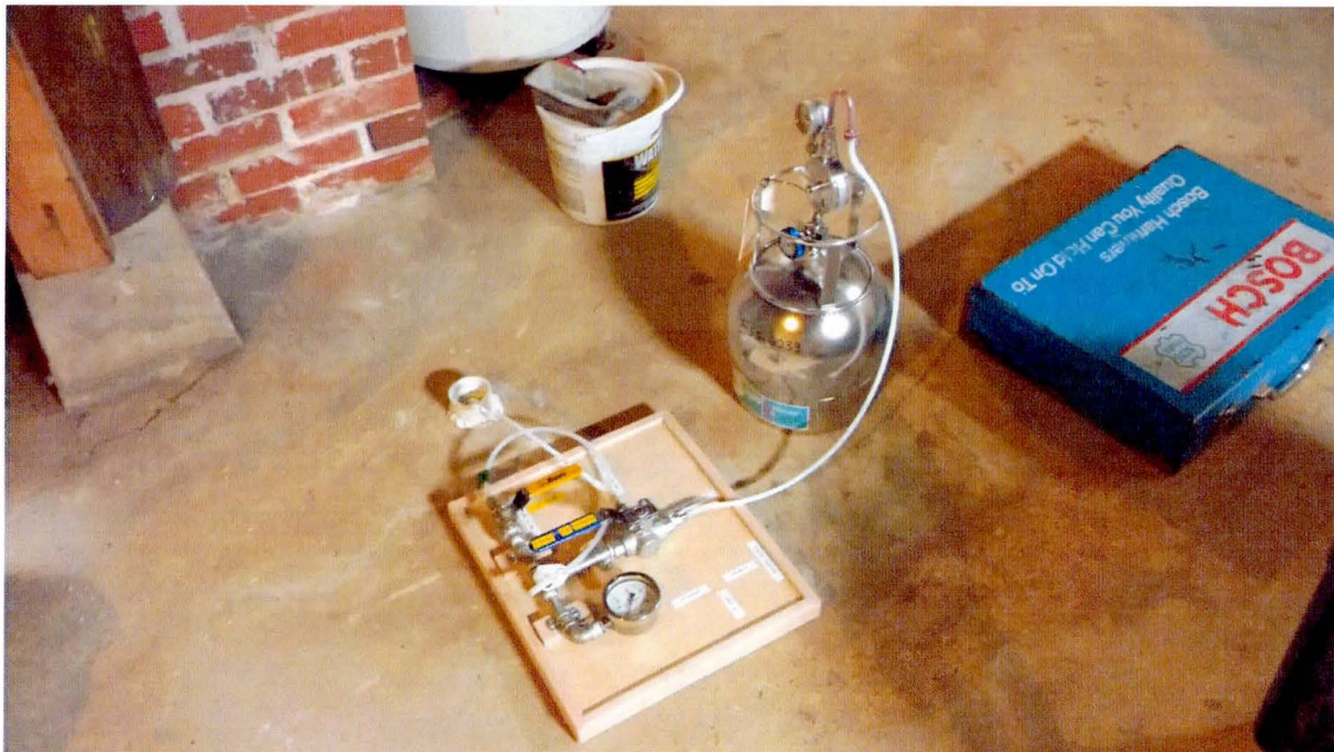
Photo 4: 920 Church Street – Sub-slab sample collection.
