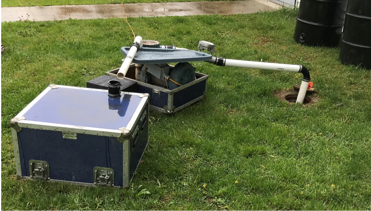
Photo 1: SVE blower for SVE pilot test set up on well SVE-2. May 3, 2021
