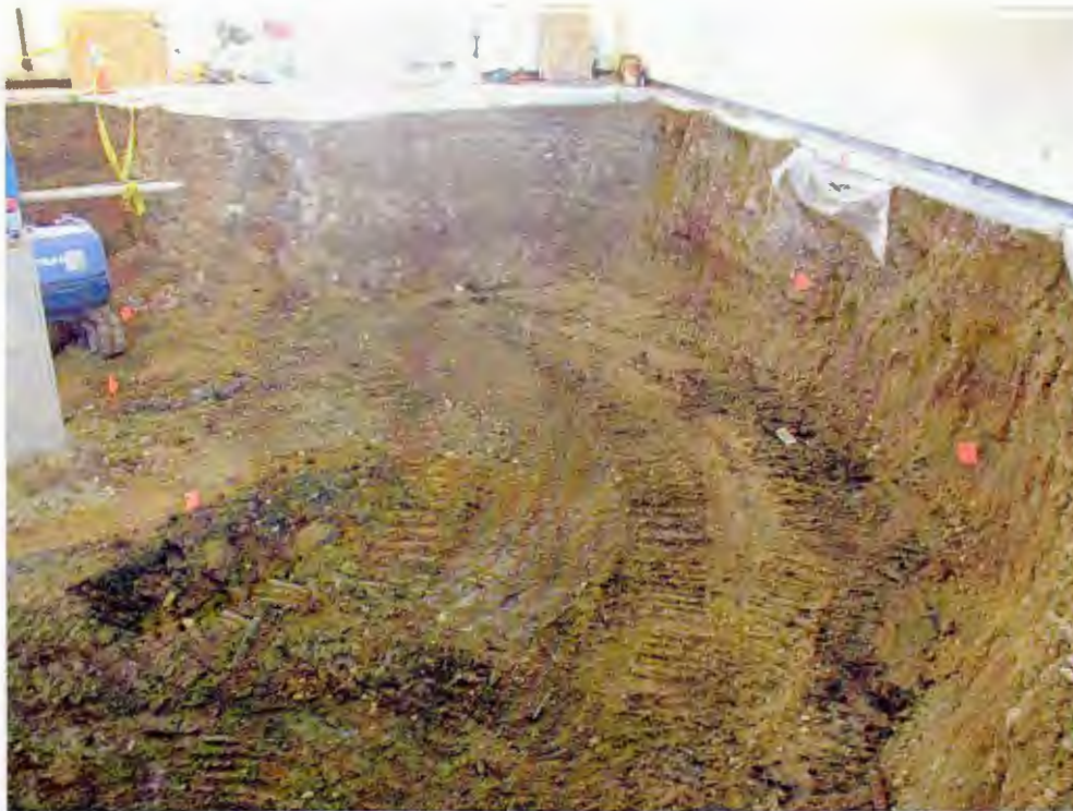
Photo 6: Orange flags were used to mark soil sample locations. View to the southwest.
