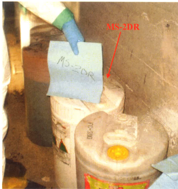
Photograph No.: 5 Photographer: Caitlin Ruza Area: Bldg V-Basement TDD Number: TO-05-10-12-0002 Contract: EP-S5-10-10, OTIE Date: January 24, 2011 Site Name & Location: Mirro-Spirtas Site, Manitowoc, Manitowoc County, Wisconsin Photograph Subject: MS-2DR was collected from the second drum back in the line of 6 drums on the basement level of Building V
