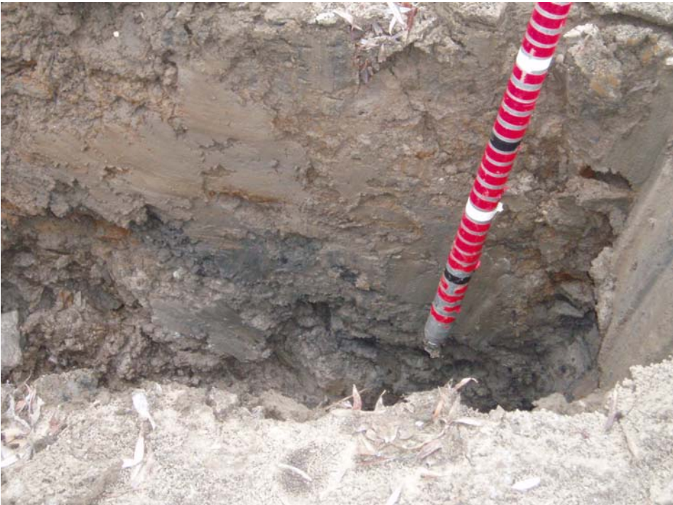
Photo #10. Test Pit #1, south end of Embayment out from retaining wall. Gray blocky material at the bottom is till.
