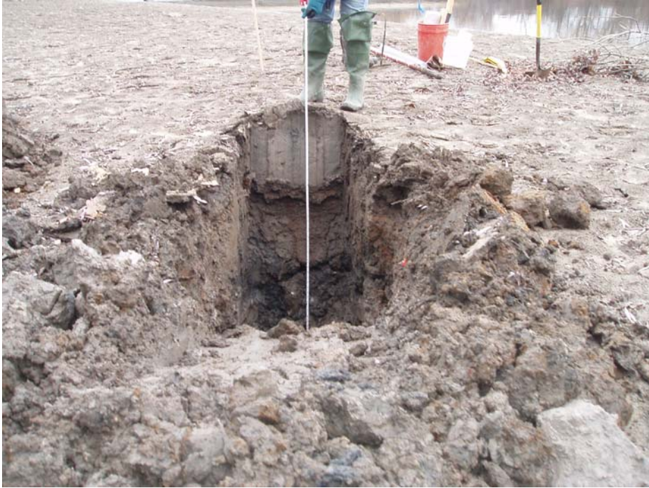
Photo #13. Test Pit #2, approximately 5 feet deep.
