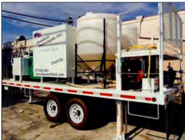
Photo 3. Deep Earth Technologies, Inc. was set up on the driveway south of the excavation and treatment area. Cool-Ox™ treatment solution was mixed in the pump truck.
