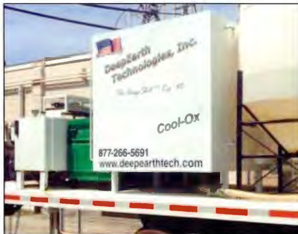
Photo 4. The patented Cool-Ox™ in-situ remediation technology utilized during the pilot test included chemical oxidation and accelerated biodegradation to eliminate volatile organic compounds in soils.
