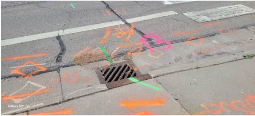
Proposed location of boring B-13 (not completed due to utilities)
