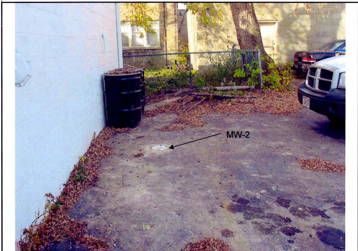
12. View groundwater monitoring well MW-2 and the 55-gallon drums containing drill cuttings and purged groundwater to the north of dry cleaner building.
