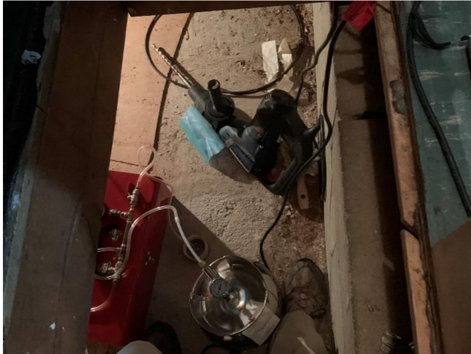
Photo #5 Subslab Vapor Sampling in crawlspace at 3119 N. 47 th Street residence.
