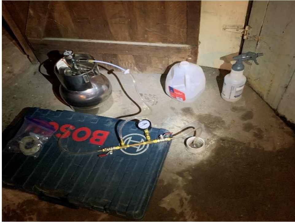
Photo #3 Subslab Vapor Sampling at 4714-4716 W. Burleigh Avenue, North Sample.
