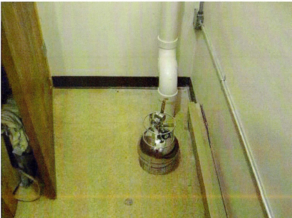
2) View of ambient air sample collection near sub-slab vapor monitoring point SS-2.
