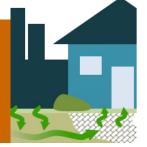
Chemicals used in commercial or industrial activities – dry cleaning chemicals, chemical degreasers and petroleum products such as gasoline – are sometimes spilled and leak into nearby soil or groundwater. When this happens, these chemicals may release gases or vapors, which travel from the contaminated groundwater or soil and move into nearby homes or businesses. This is called vapor intrusion.
