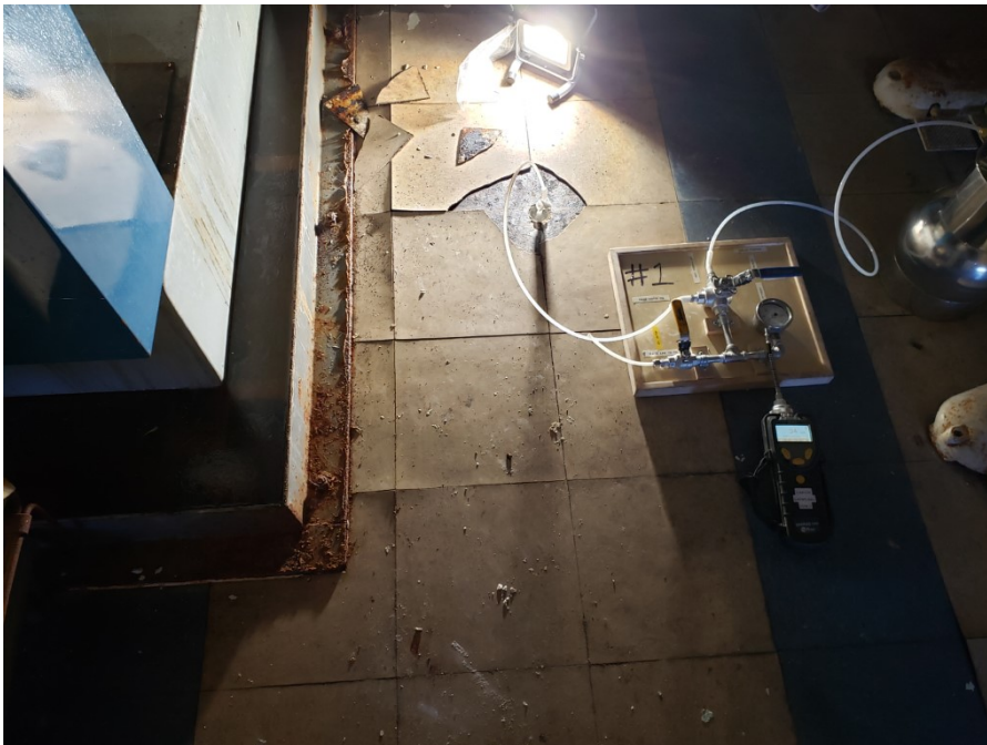
Photo 6: Sub-slab sample SB-1 in progress at 711 S. Church St., adjacent to liquid-filled containment around dry cleaning machine (9/18/20).
