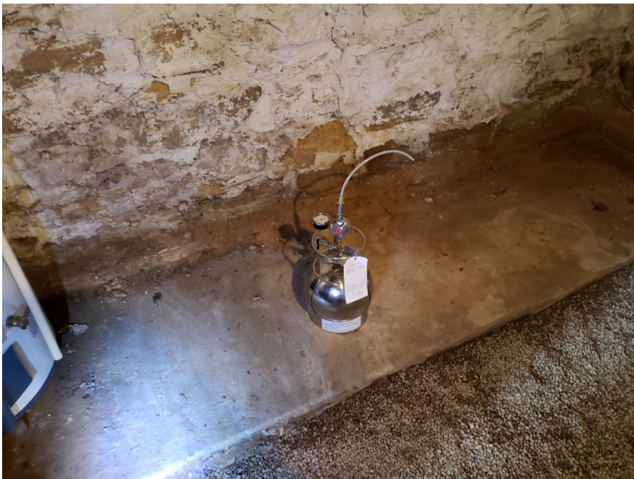
Photo 4: Air ample IA-3 in progress in basement of 735 Sextonville Rd., looking southwest (9/17/20).
