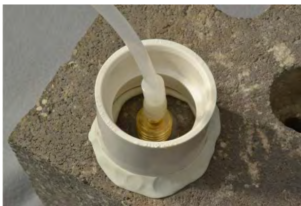
Figure 6. Water dam used for leak detection.
